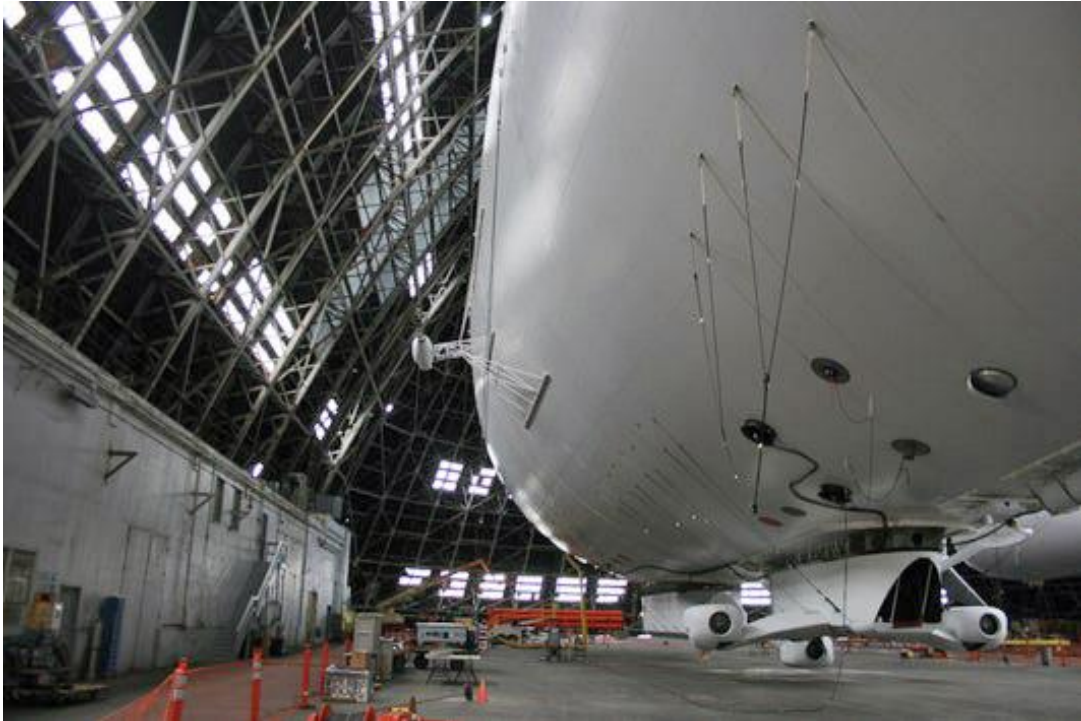
Rear quarter view of the M1400 airship prototype floating in its hanger. The power car (the aft gondola), with three diesel engines, is in the foreground. One of the flank-mounted vectorable turboprop engines can be seen attached near the mid-plane of the hull.
