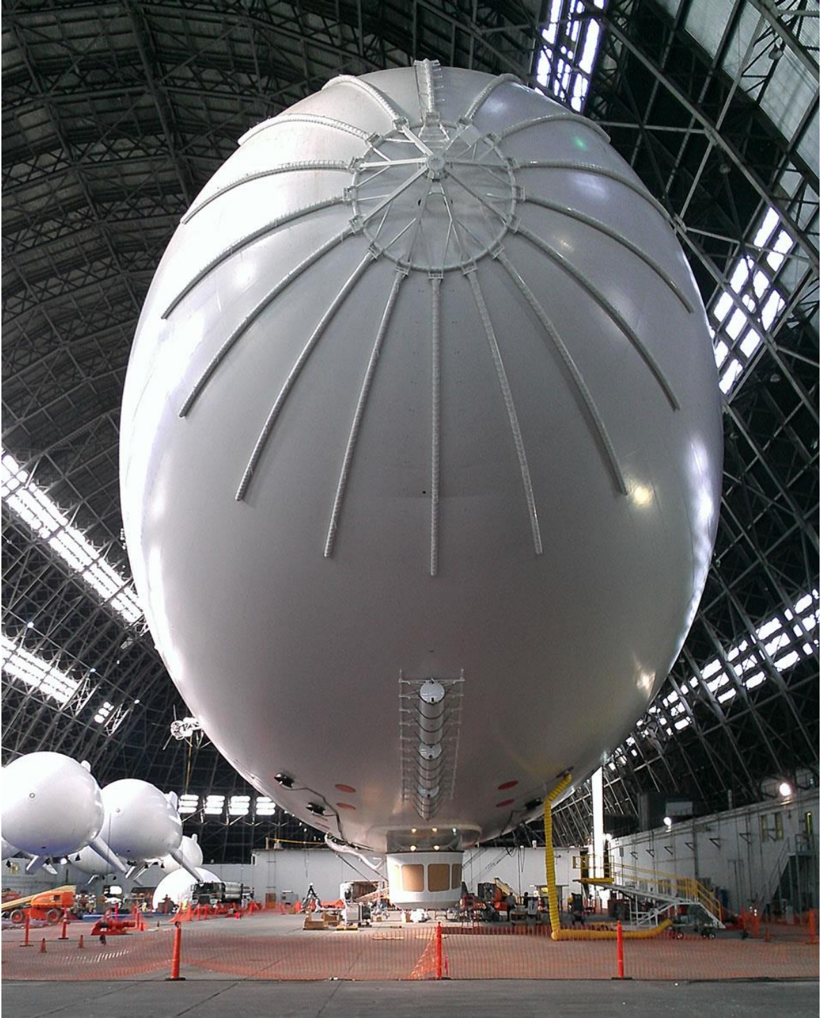
Front view of the M1400 airship and the control / payload car (the forward gondola). Source: Mav6
