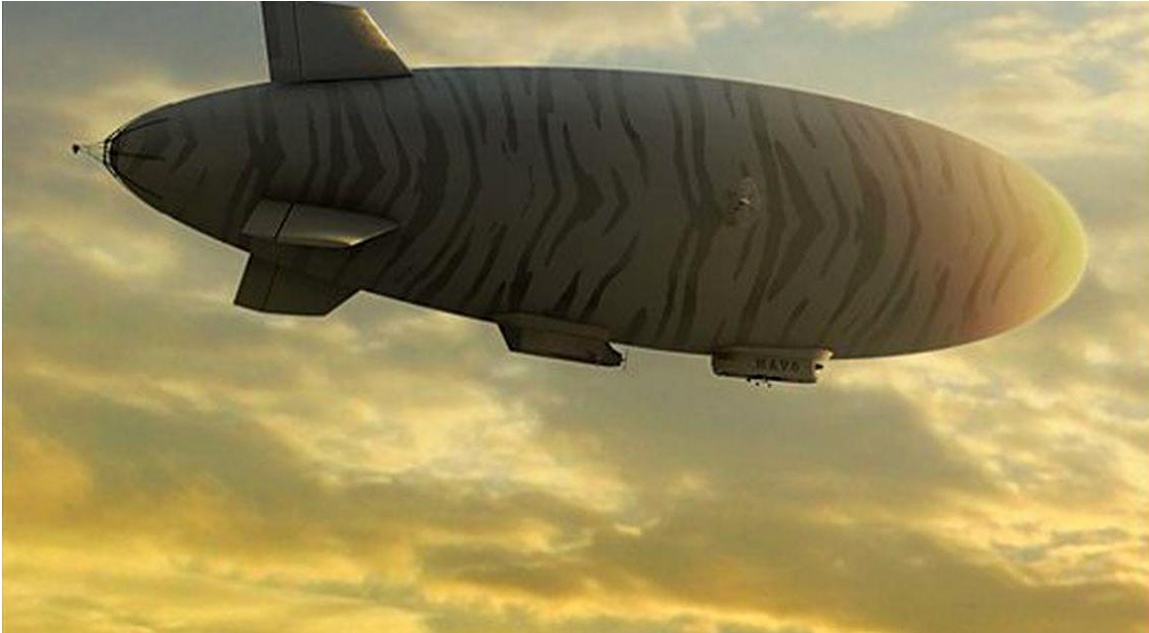
Artist's concept of an operational Blue Devil Block 2 airship showing the two under-slung gondolas. Source: Mav6
