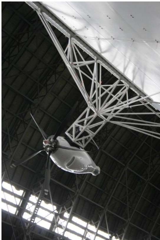
One of two vectorable turboprops engines mounted amidships via a structural framework that distributes loads into the fabric hull. Source: David Axe via Wired 6 Jul 2012
