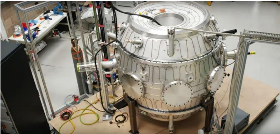
External view of the inner vacuum vessel for the ST40 spherical tokamak. Source: Tokamak Energy
