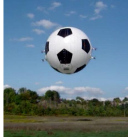
Left: This appears to be a four-engine adaptation of the AS-62 Aerosphere configured as a soccer ball and being prepared for launch. Source: Jeremy Gutsche via TrendHunter, 27 March 2006;
