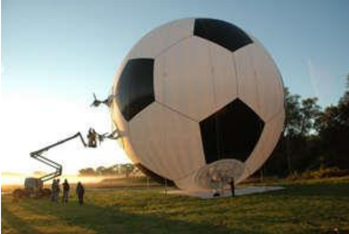
Left: This appears to be a four-engine adaptation of the AS-62 Aerosphere configured as a soccer ball and being prepared for launch. Source: Jeremy Gutsche via TrendHunter, 27 March 2006; Right: Soccer ball in flight. Source: Screenshot from video.
