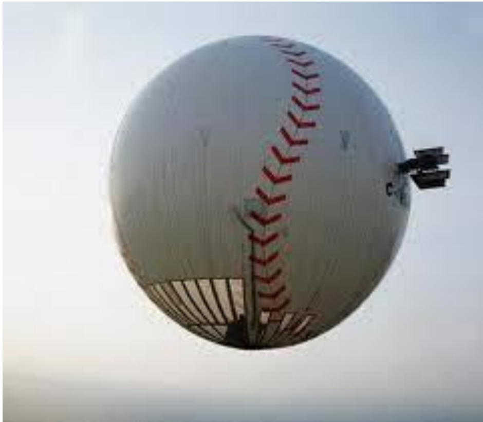
SPAS-4 in 1996 painted as a baseball for the Atlanta Braves baseball team and the Atlanta Olympics. Note the interior cockpit at the bottom of the sphere. The port engine and slipstream deflector vanes are a prominent feature at the “equator” of the spherical envelope. Source: Pinterest
