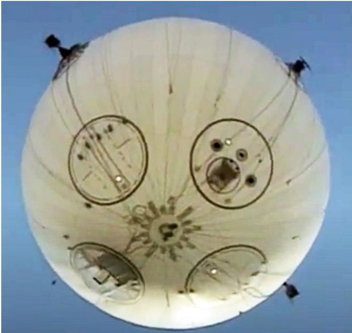
Above: View of the AS-62 as it flies overhead, showing the two flank propulsors and the pusher propulsor on the rear hemisphere.
