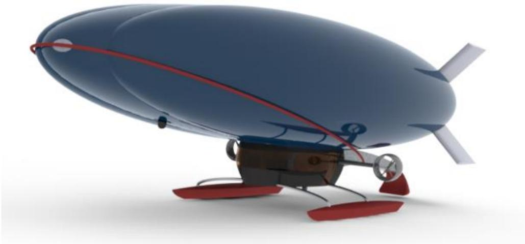
*Rendering of the A-N1800 airship with tri-lobe envelope and floats for water landings. Source: A-NSE*
