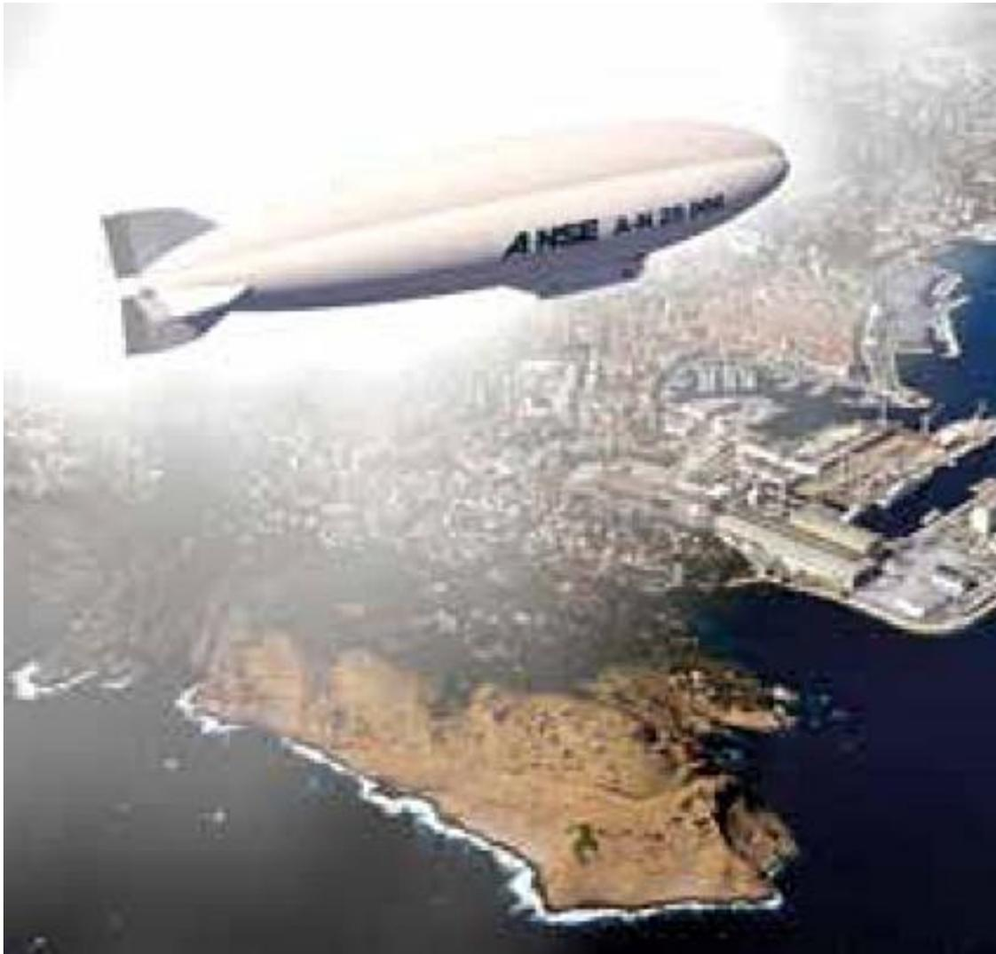
*Rendering of the A-N 20 000 medium-lift airship concept with tri-lobe envelope. Source: Aerall.org*
