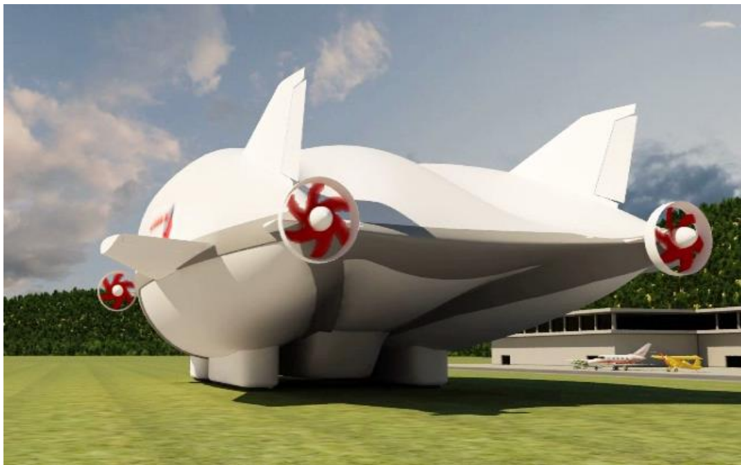
Rear quarter view of the Aerocat R12 concept shown on the ground, with ACLS extended. Source: AeroVehicles.
