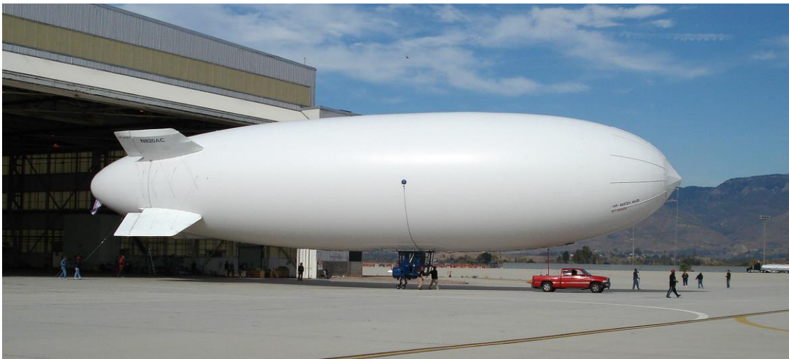
The first component of the G2R was based on an Aeros 40D Sky Dragon blimp. Source: Aeros
