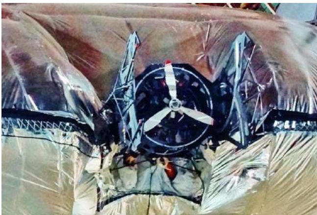
Stern-mounted, fixed engine & 3-bladed propeller with thrust-vectoring "paddles" to divert the propeller slipstream (to vector thrust). Source: Aeros
