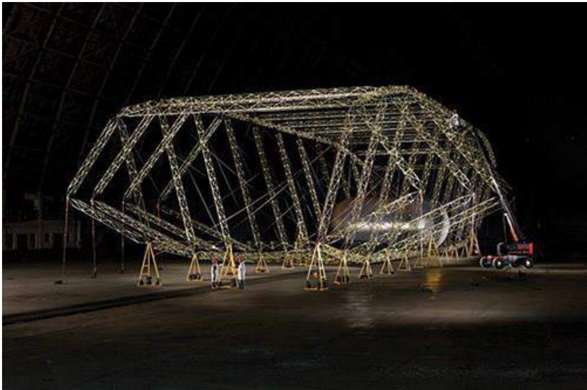
The Dragon Dream's lightweight main frame, which supports the airship's COSH equipment, its cockpit, cargo, and cargo containment structures.
