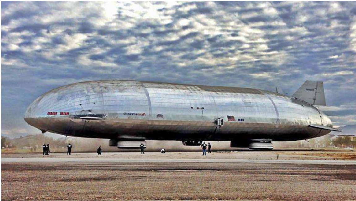
Dragon Dream outdoor taxi test on its air bearing landing system (ABLS). Source: Aeros (2013)
