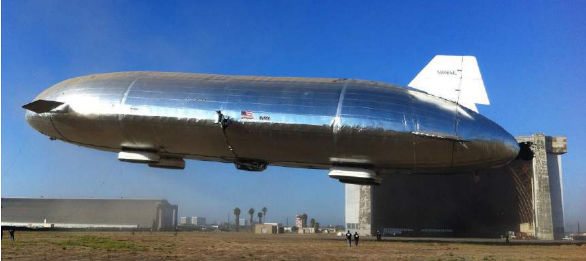
Dragon Dream flight test, September 2013. The cockpit is visible amidships, under the gas envelope. Source: Aeros
