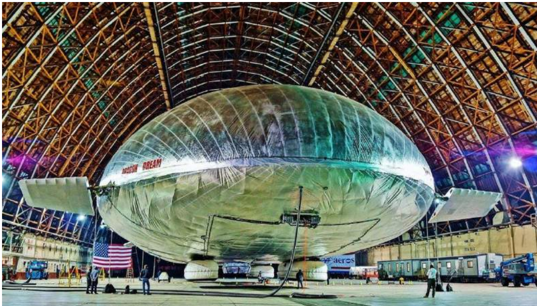
Dragon Dream bow view on first “static float test” in January 2013 (above); stern view showing the fixed aft propulsor and diverter flaps (below).
