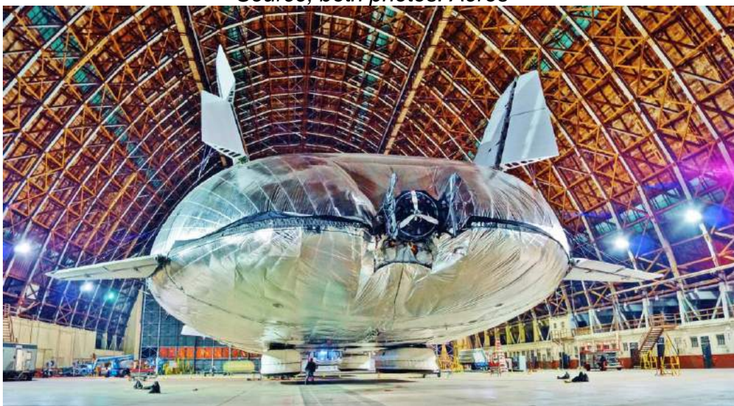
Dragon Dream bow view on first “static float test” in January 2013 (above); stern view showing the fixed aft propulsor and diverter flaps (below).
