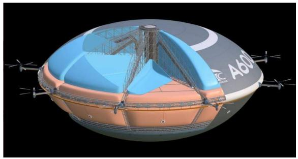
A600 cut-away drawing showing the primary internal structures: the central support column, the radial bracing trusses, and the circumferential torus ring, which supports the propulsion units. The lifting gas cells (blue) and the hot air cells (ochre / reddish color) are installed in the sectors between the bracing trusses. Source: AIDBA (2021)
