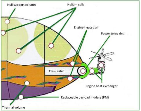
Internal details showing the engine and heat exchangers in the hot air supply system. Source: adapted from AIDBA
