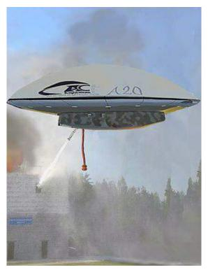
The 20-metric ton (22-ton) payload A20 will be the prototype for the entire Aerosmena family. This 70-meter (230 ft) diameter utility aeroplatform can be configured for a variety of missions, such as:
