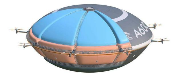
A600 with the outer shell pulled back to show the placement of lifting gas cells (blue) and the hot air cells (ochre / reddish color). Source: AIDBA (2021)
