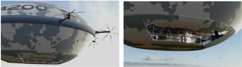
A200 drone bay door opening (left) and drone launch from internal drone bay (right).
