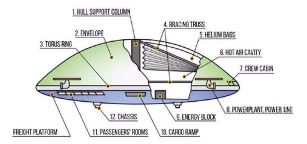
General arrangement of an Aerosmena aeroplatform. The rigid hull structure includes the central hull support column, the torus ring around the periphery & the internal bracing trusses. Source: AIDBA
