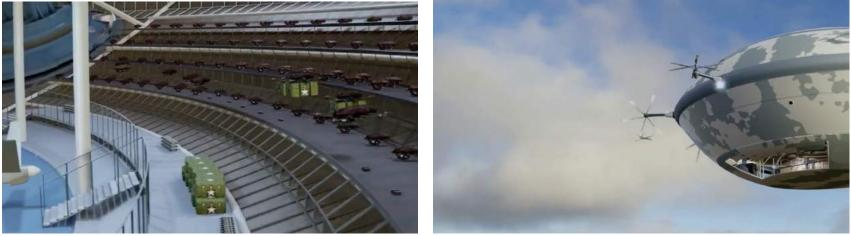
A200 internal drone bay details (left) and drone recovery (right). Source, all graphics: Screenshots from 2021 AeroCrat video
