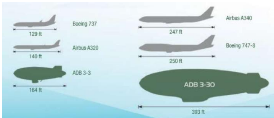
Relative sizes of the ADB 3-3 and the larger ADB 3-30 cargo airship. Source: Airship do Brasil
