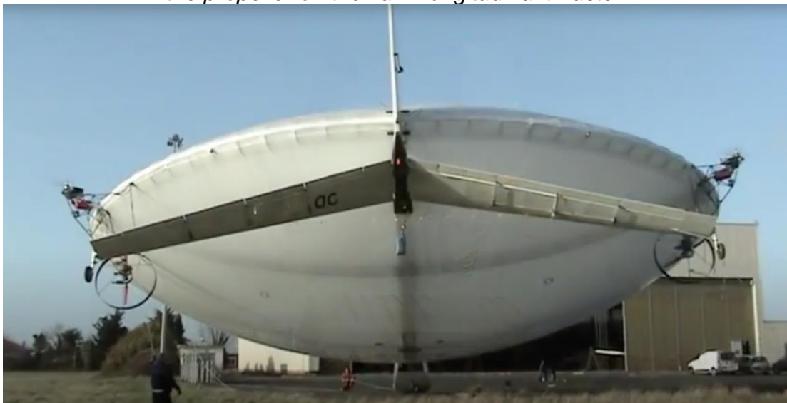
Stern view showing the tail aerodynamic surfaces and the placement of the flank compound thrusters. Source, two photos: Screenshots
