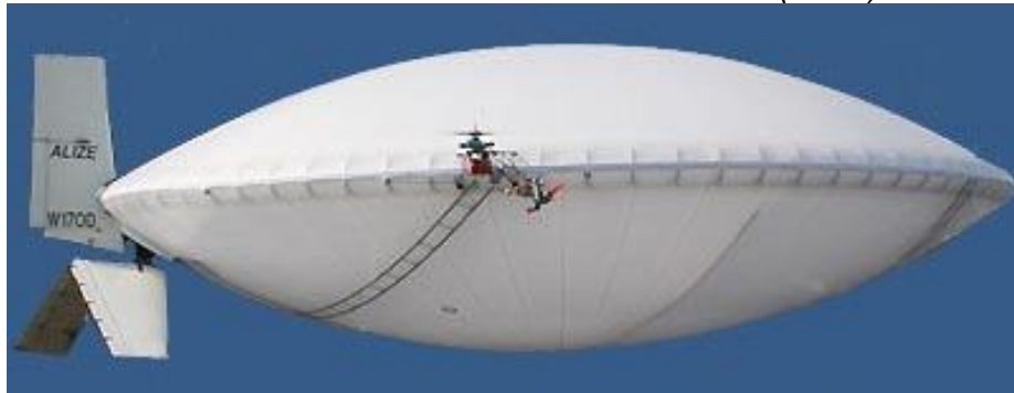
Alizé first flew by remote control, without the cockpit gondola installed. Source: LTA Solutions (2015)
