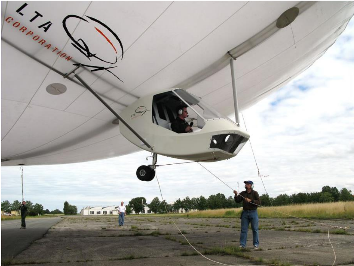
Alizé with enclosed cockpit. Note that the cockpit's support struts connect directly to the rigid framework of the hull.
