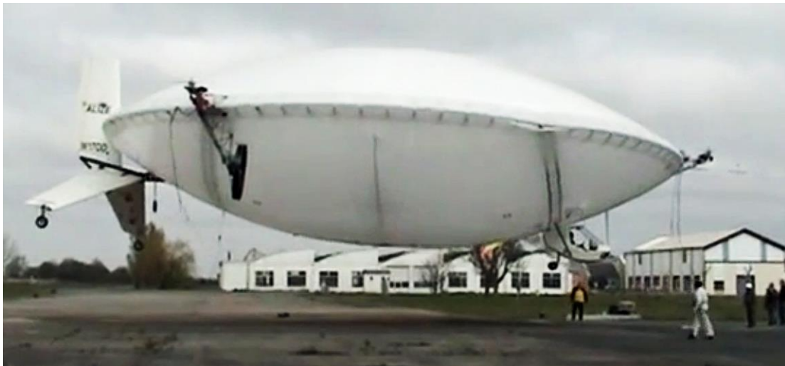
Profile view showing the placement of the bow and flank compound thrusters. Note the short duct surrounding the propeller on the flank longitudinal thruster.
