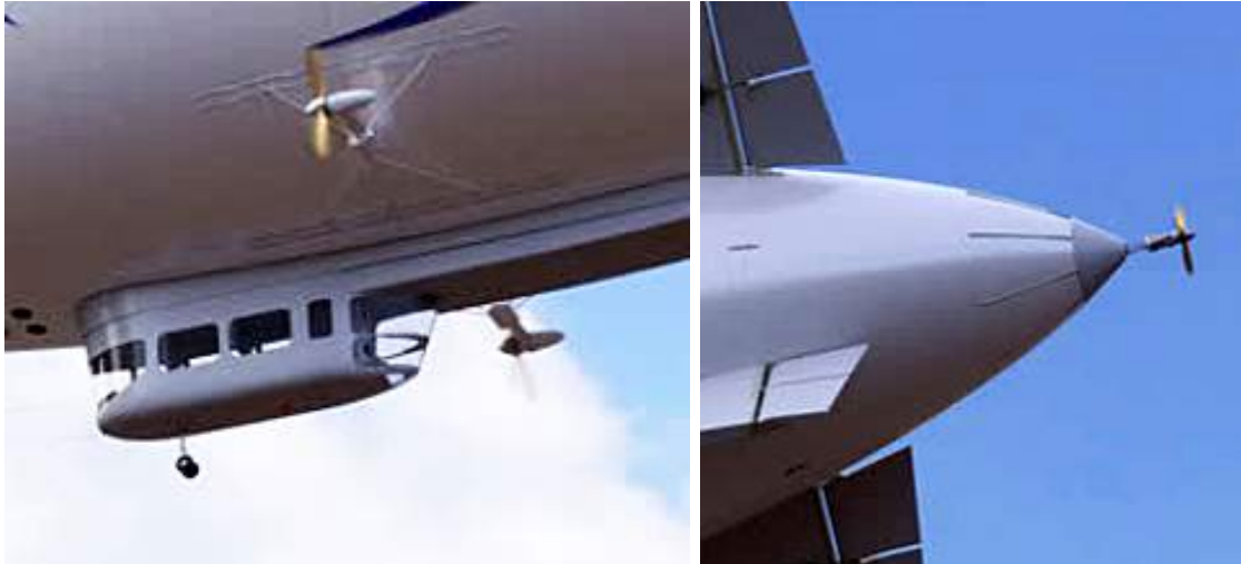
Rendering of Atlas-6 gondola & flank vectoring propellers (left) & the stern vectoring propeller (right). Source: Atlas
