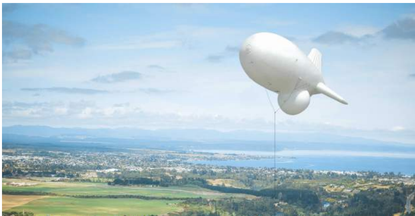
Rendering of a Large Volume TA configured as a radar platform for an airborne early warning system. Source: Atlas
