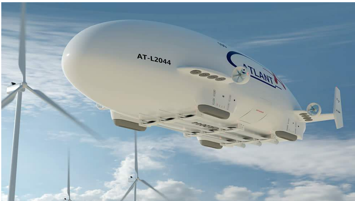
ATLANT 100 with external belly cargo trays carrying a set of wind turbine blades. Source: Atlas
