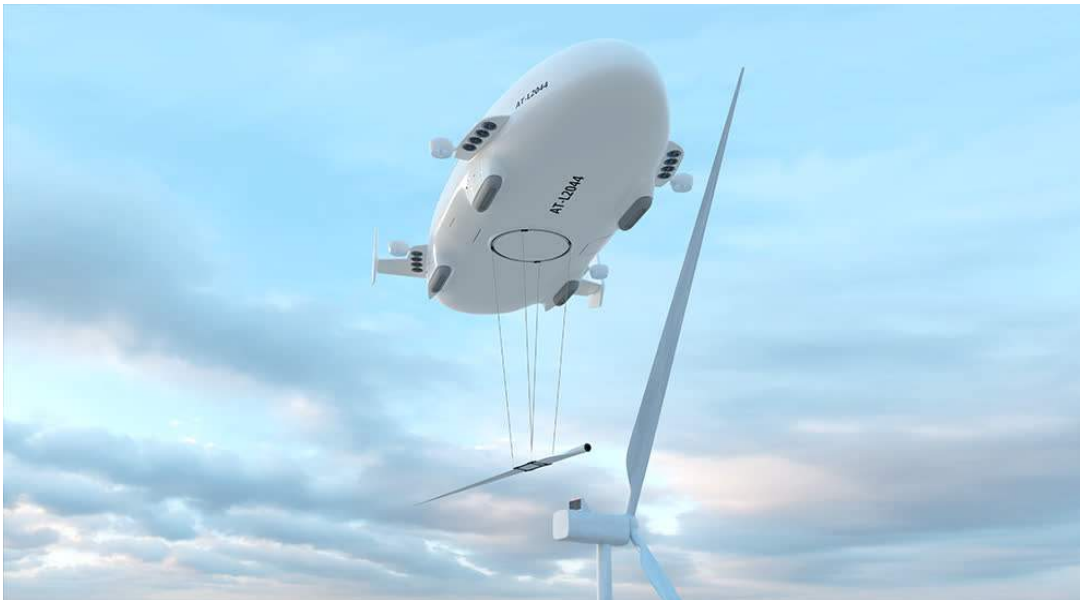
ATLANT 100 with rotating load platform operating as a flying crane carrying a single suspended wind turbine blade. Source: Atlas
