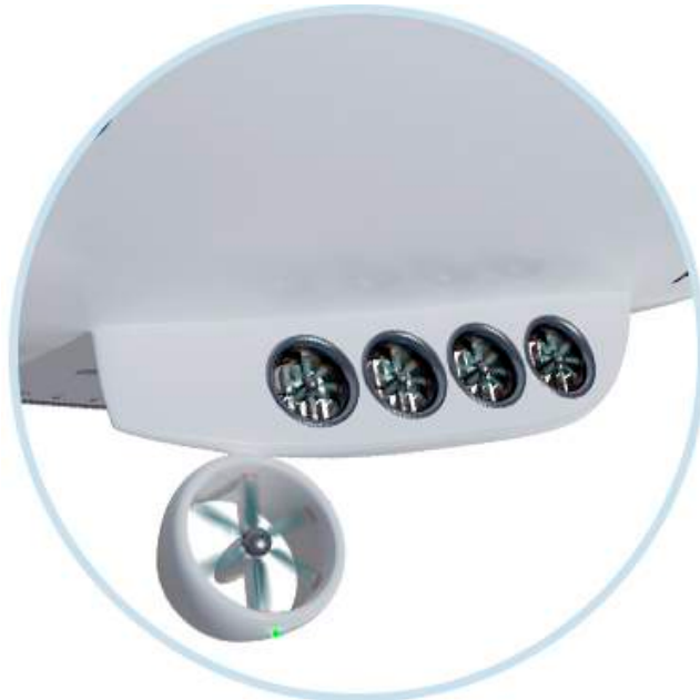
One of four MDM + ALM installations on an ATLANT-30. Source: Atlas
