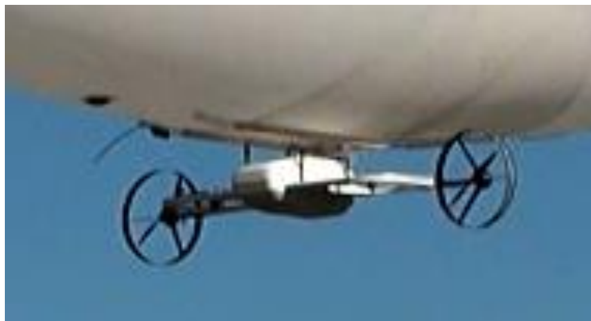
The gondola and shrouded, electric motor driven vectorable propulsors attached to hard points on the bottom of the envelope.
