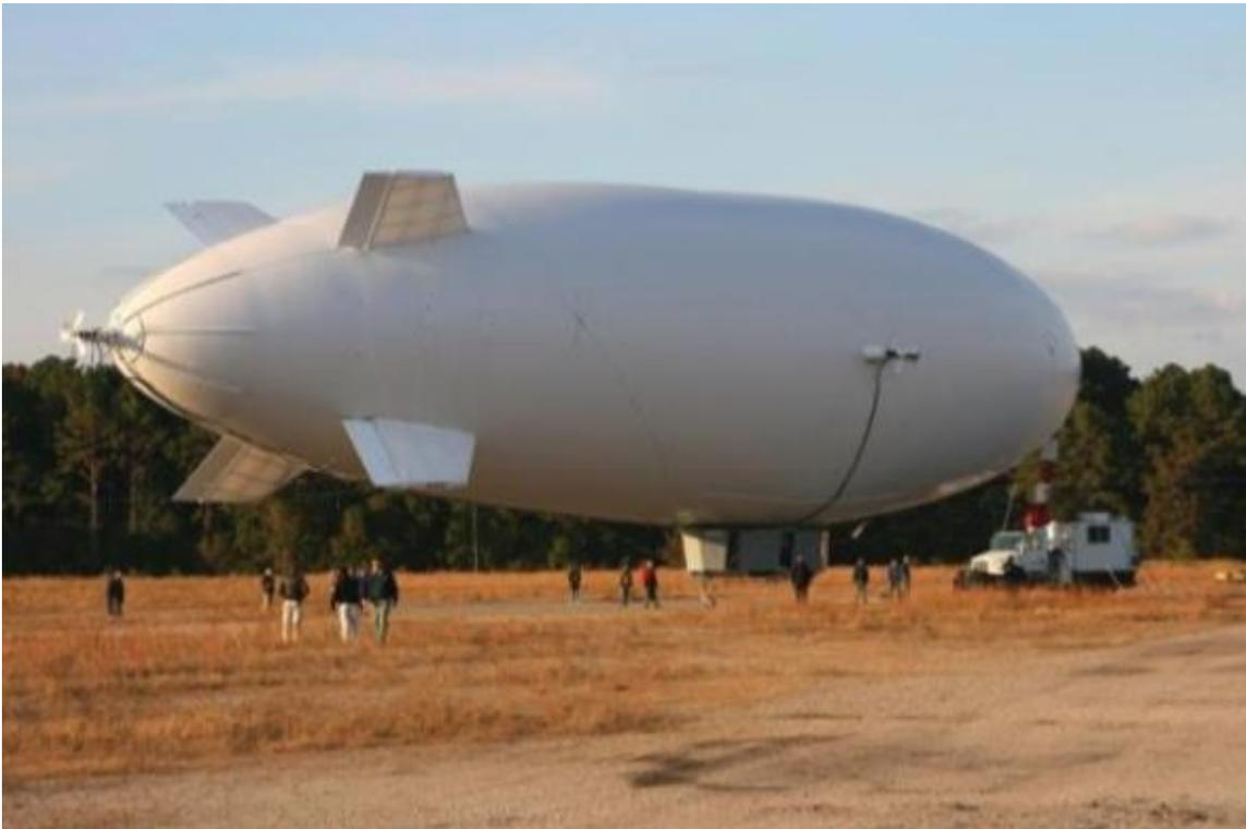
*Polar 400 airship. Note the hydraulic lines run externally to the flank-mounted hydraulically-driven propulsor. Source: Guardian*
