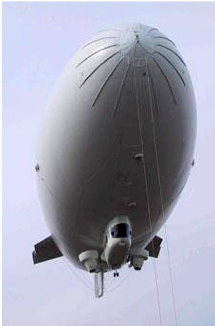
*Airships Industries Skyship 600 with Lycoming IO-540 vectored thrusters. Source: Guardian Flight Systems*
