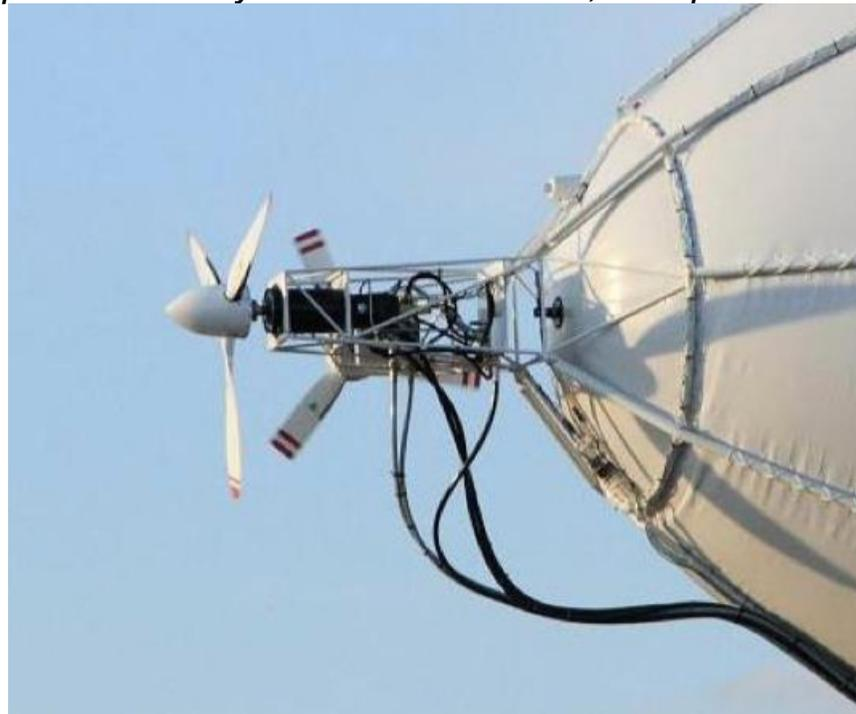
**Propulsor arrangement:** The Polar 400 propulsor arrangement is very similar to that of the Zeppelin NT with two flank-mounted vectorable propulsors at the envelope mid-plane and two aft propulsors, one providing thrust and one providing lateral thrust. A key difference is that the Polar 400's aft engines are both fixed, while the Zeppelin NT's aft longitudinal propeller can be vectored 90° down for lift and pitch control.
