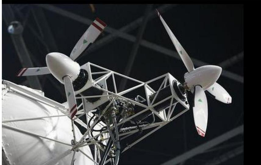
*Tail mounted hydraulically-driven fixed propellers mounted to the envelope. Note the hydraulic lines. Source, both photos: Guardian*
