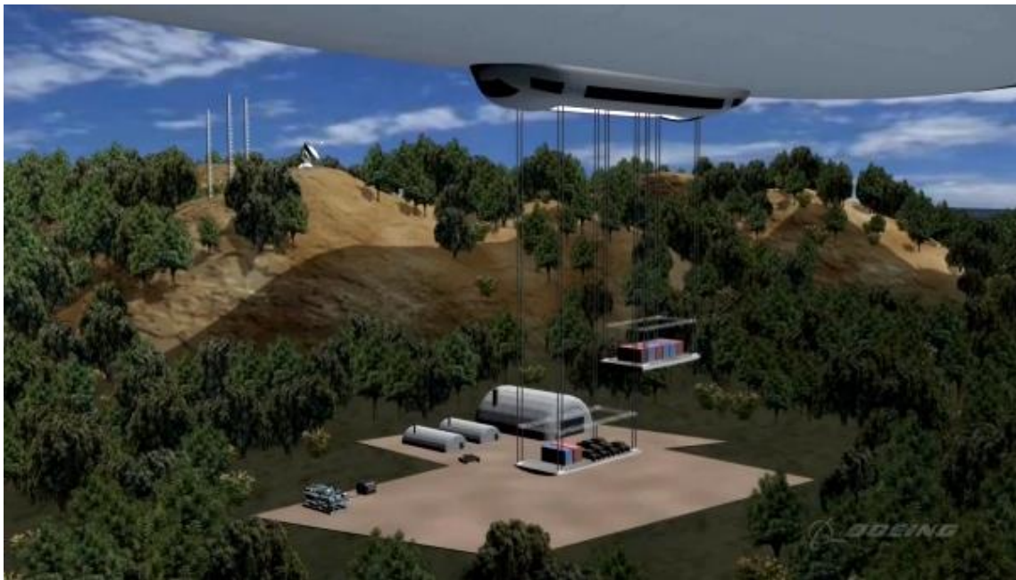
A depiction of Boeing's Hybrid Thermal Airship making an in-flight load exchange. Source: Boeing via Todd Bishop/GeekWire (2011)
