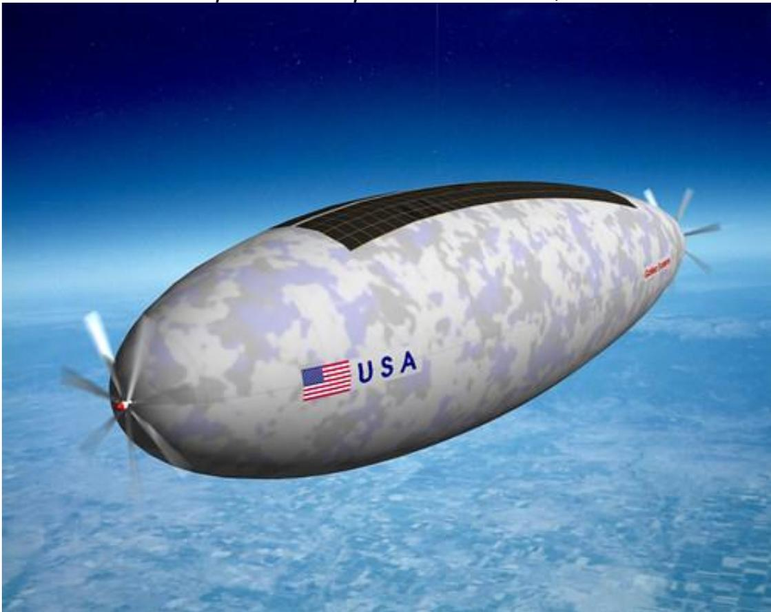
*General configuration of a similar US concept for a solar-powered stratospheric airship, circa 2000. Source: DARPA*
