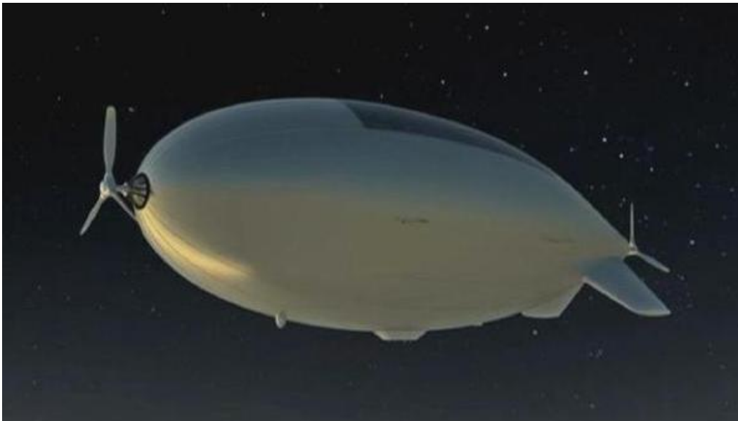
General configuration of China's Yuanmeng (Dream) solar-powered stratospheric airship. Source: CNTV, China
