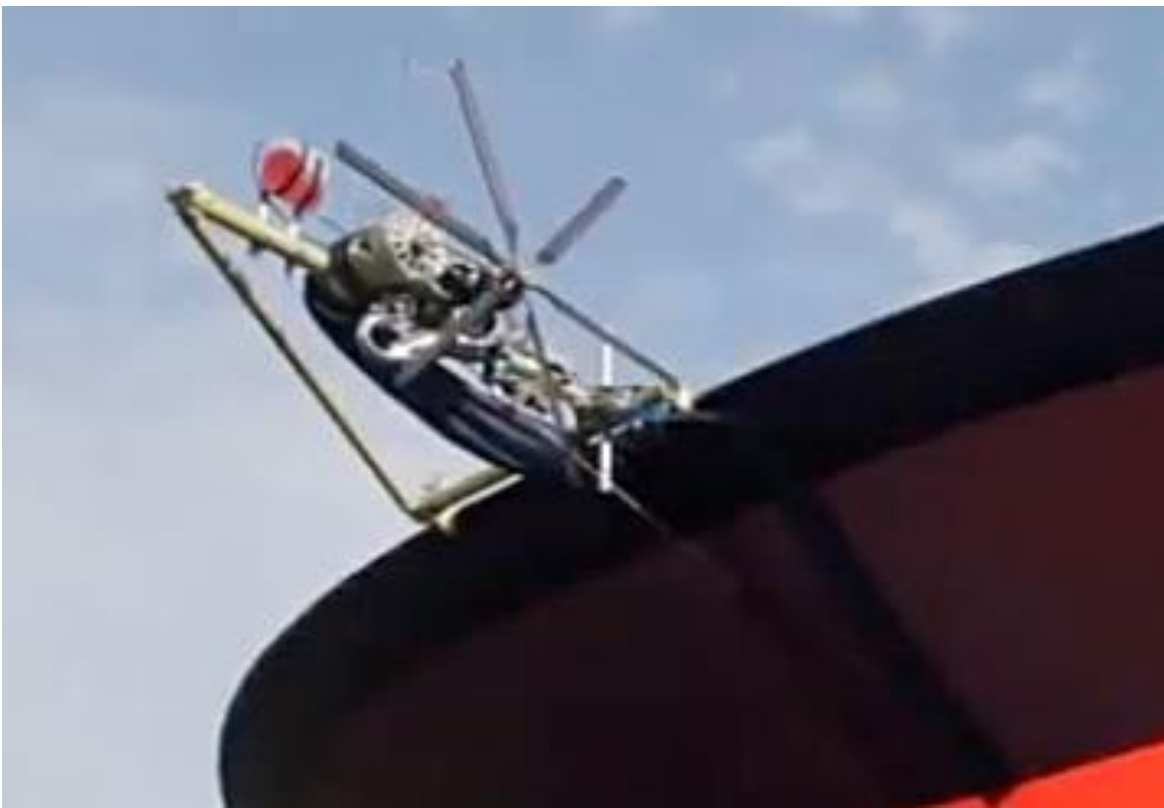
DP-27 vectoring propeller (1 of 4). Source: DDBA
