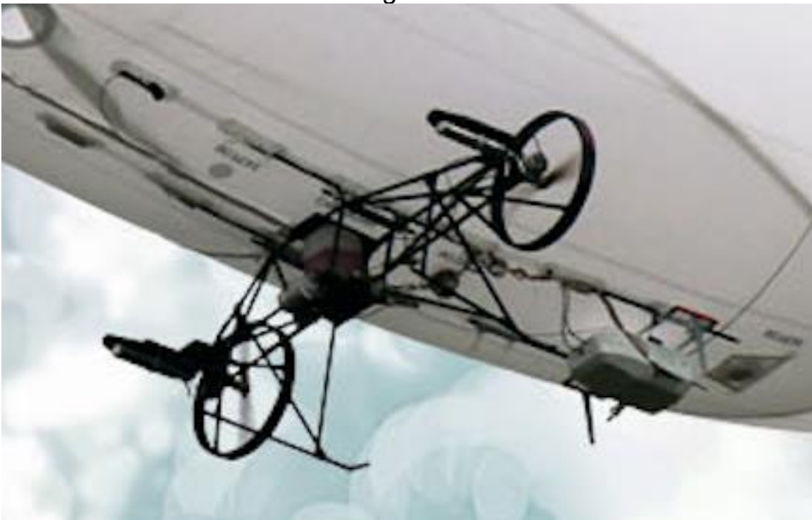
Close-up of DP-29 propulsion and payload modules. Source: DDBA
