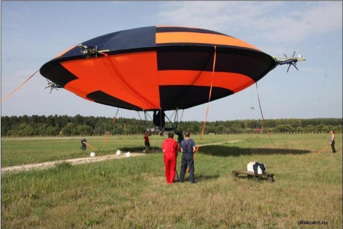
DP-27 tethered with gondola exterior skin removed. Source: DDBA
