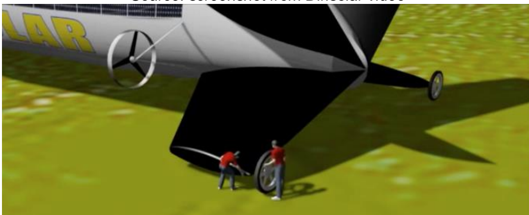
Wheels attached to the rear stabilizers after landing allow the airship to “weathervane” into the wind. Source: screenshot from Dirisolar video
