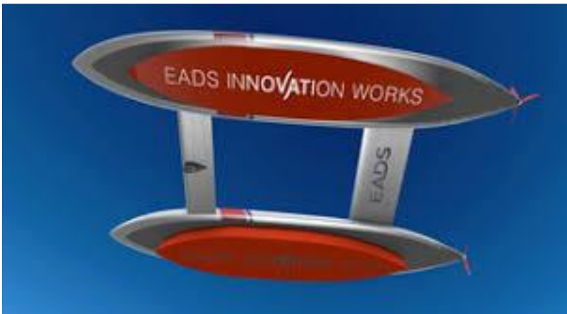
View from below, multi-segmented buoyancy cells retracted.
