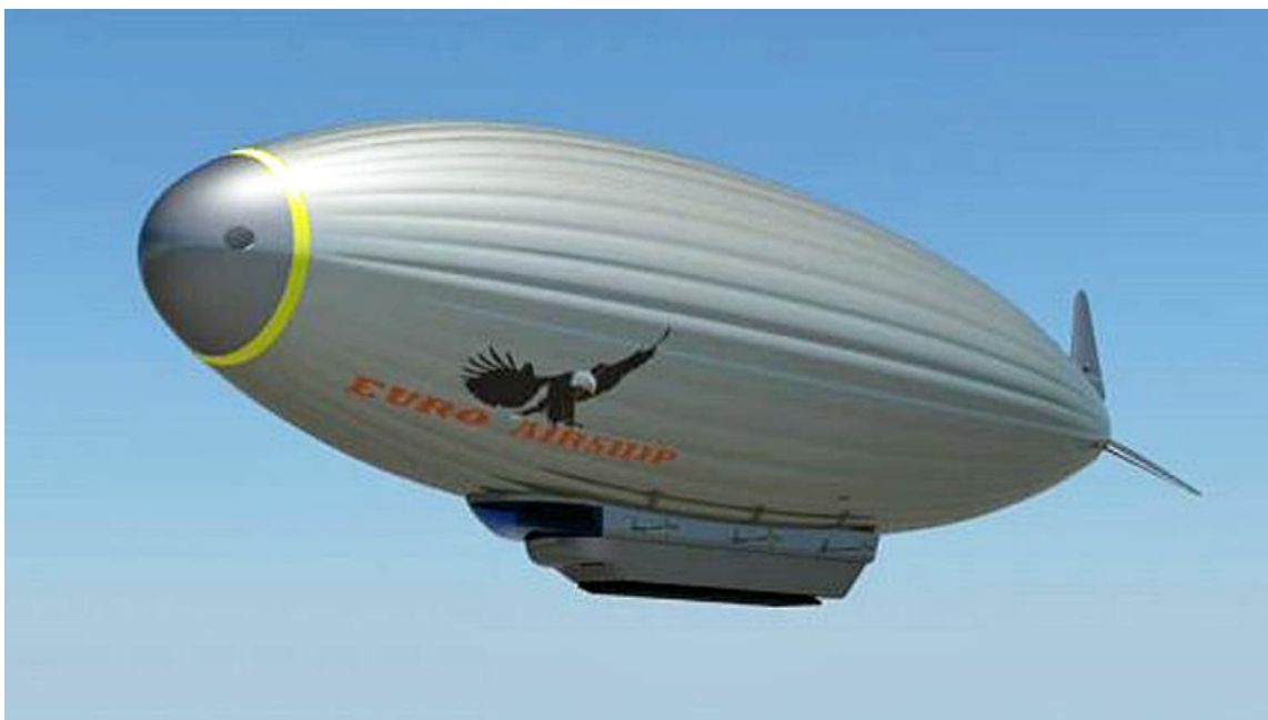
Front quarter view of a DGPatt airship. Note the placement of the bow lateral thruster on the nose cone and the propulsion propellers along the side of the gondola. Source: Euro Airship
