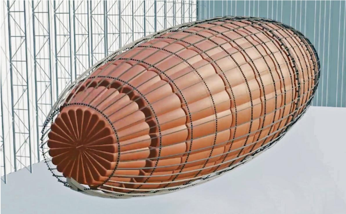
Rendering of Solar Airship One showing the helium gas cells (brown) inside the rigid airframe, which has two reinforced transverse hull frames that support the flank-mounted propellers & propulsion system loads.
