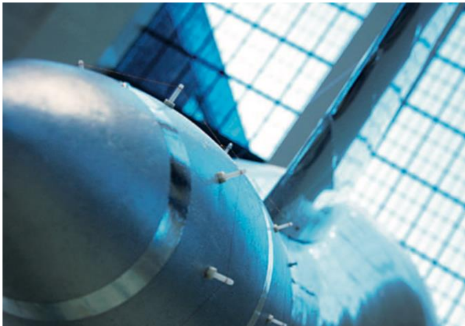
The Airfish electrostatic ionic jet on the tail cone. Source: Festo AG & Co. KG
