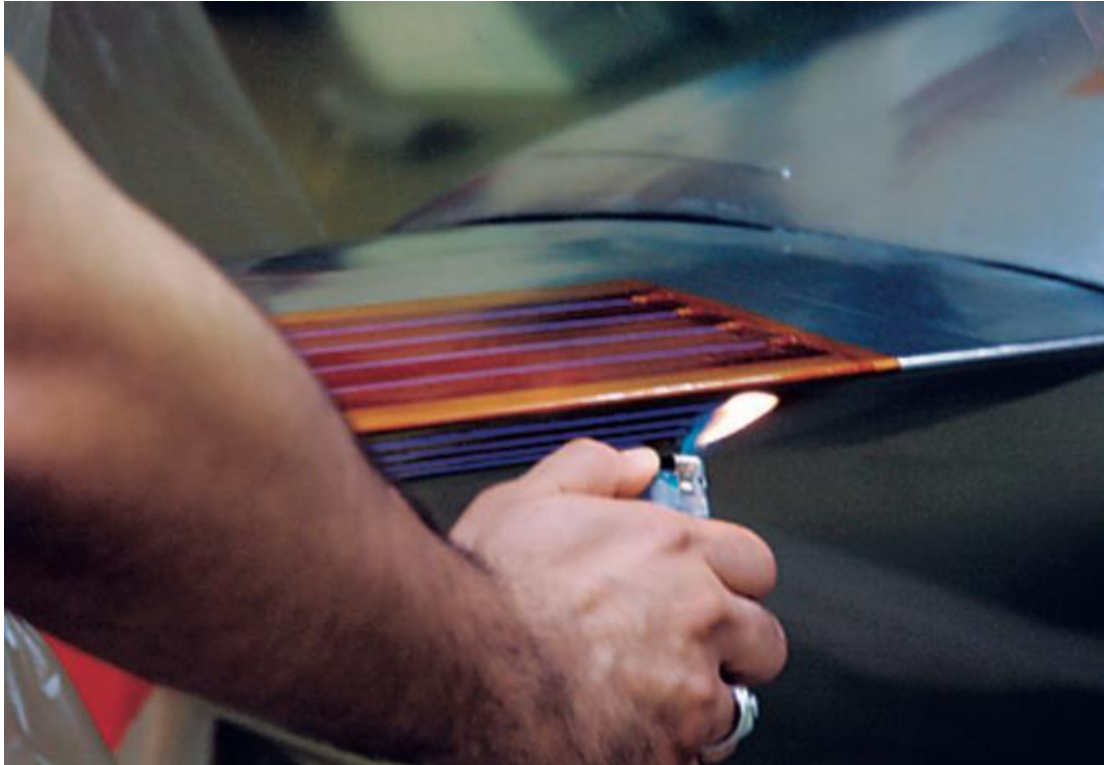
The Airfish plasma ray on a side wing demonstrating the propulsive airflow deflecting the flame of a cigarette lighter Source: Festo AG & Co. KG
