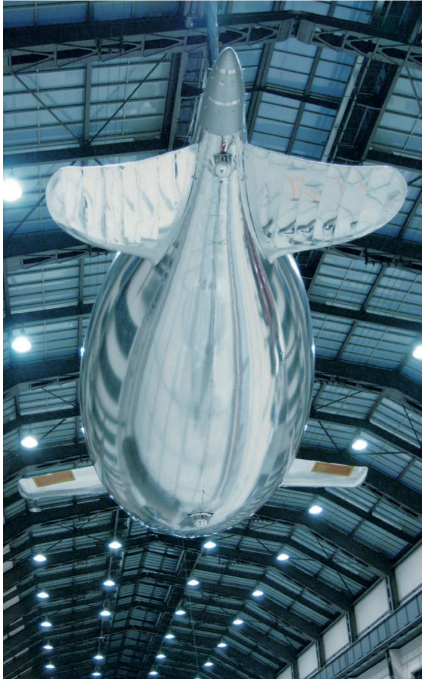
Airfish overhead. Note the plasma ray panels inset on the side wings. The electrostatic ionic jet is on the tail cone. Source: Festo AG & Co. KG
