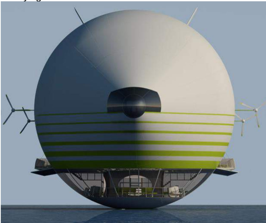
The pilot station is in the nose of the craft. Note the four propellers and the open-air balcony above the stub wings and the pressurized passenger deck at the bottom of the hull. Source: octuri.com
