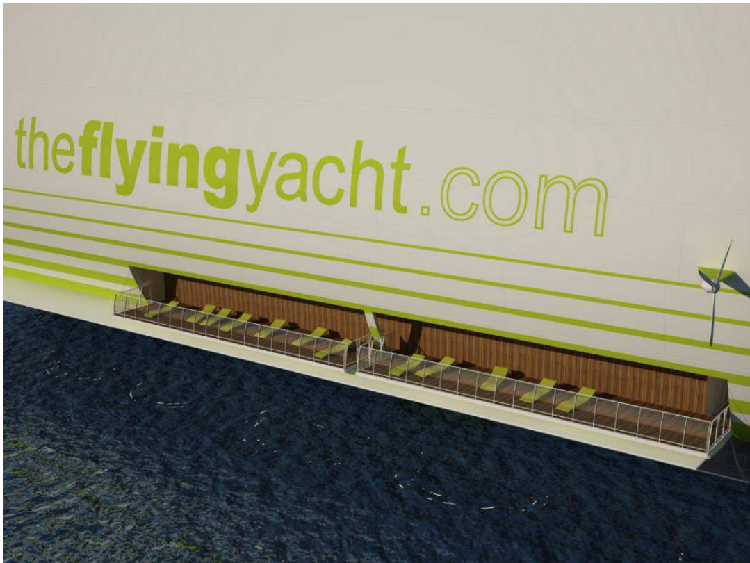
Open-air balconies above the flank wings are deployed when the Flying-Yacht is on the water. Source, both graphics: octuri.com
