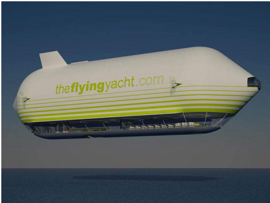
Rendering showing the general configuration of a Sky-Yacht, with the passenger deck below the helium gas envelope. Source: octuri.com
