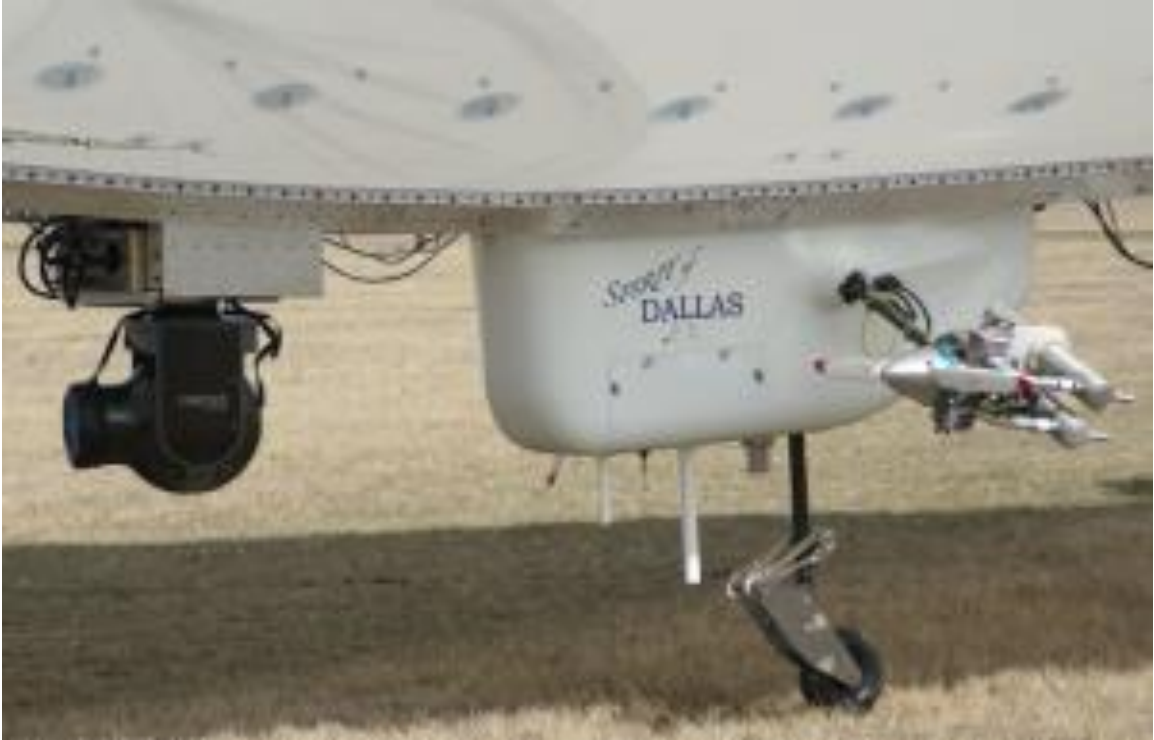
Cineflex gimbale camera mount and gondola with thrust-vectoring propellers in the horizontal cruise position. Source: GUS
