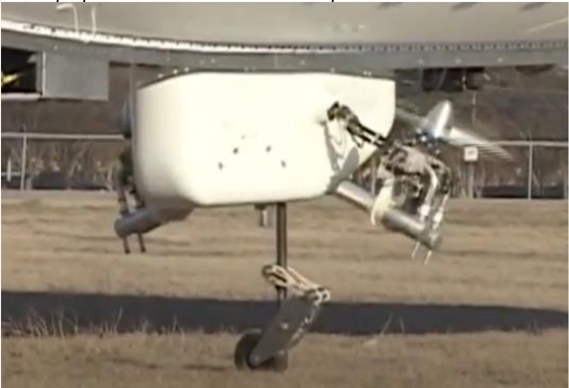
GC-75 propellers vectored "up" for vertical takeoff. Source: GUS
