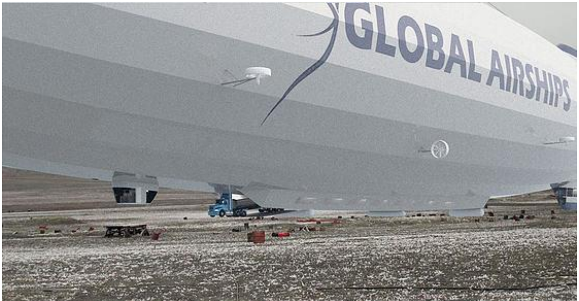
The ventral crew cabin located forward of the mid-ships cargo hold contains the forward-facing piloting station and the rear-facing crane operator station. Source: Global Airships
