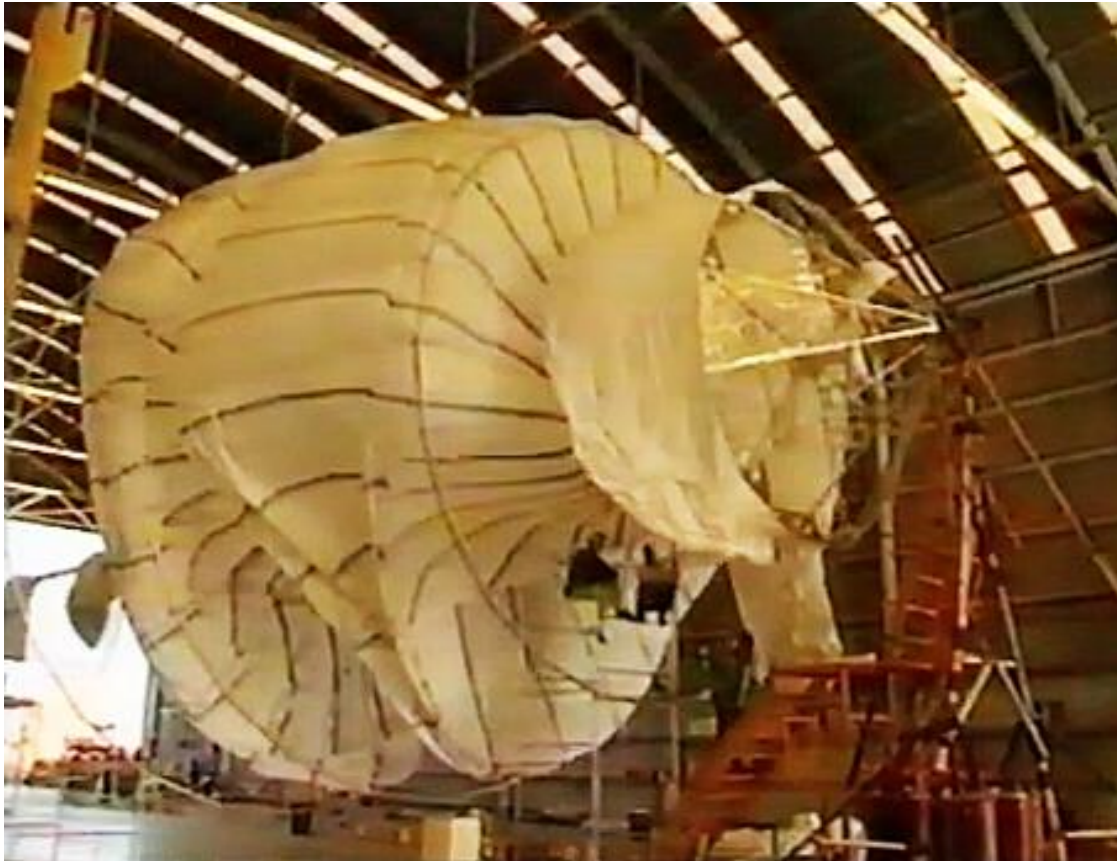
The HA-44 cockpit (right) and the helium gas bag for the first modular unit. Source: Screenshot from THAC video
