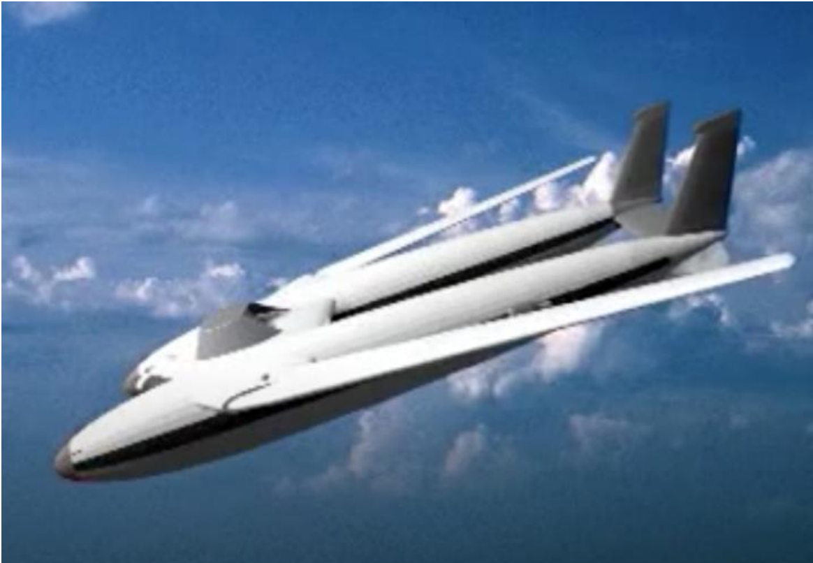
Gravity Plane descending at a steep angle with the wings highly swept. Source: Screenshot from Hunt Aviation video.
