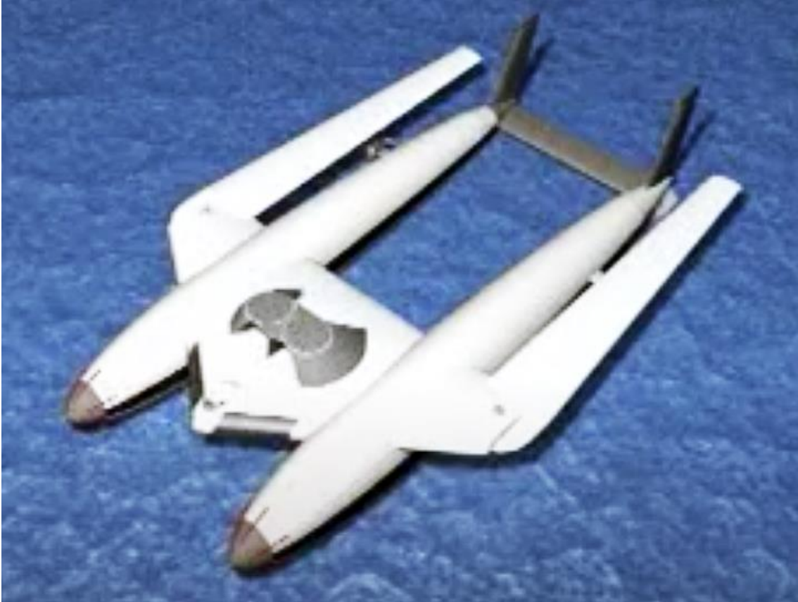
Gravity Plane landed on the water with the wings fully swept. Source: Screenshot from Hunt Aviation video.
