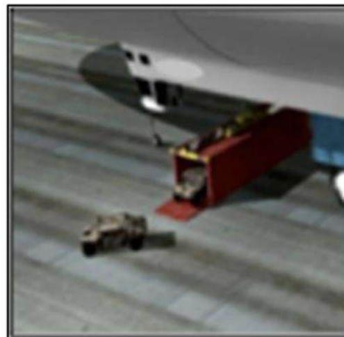
ISO cargo module handling on an LTA-70. Source, three graphics: LTA Aerostructures (2015)
