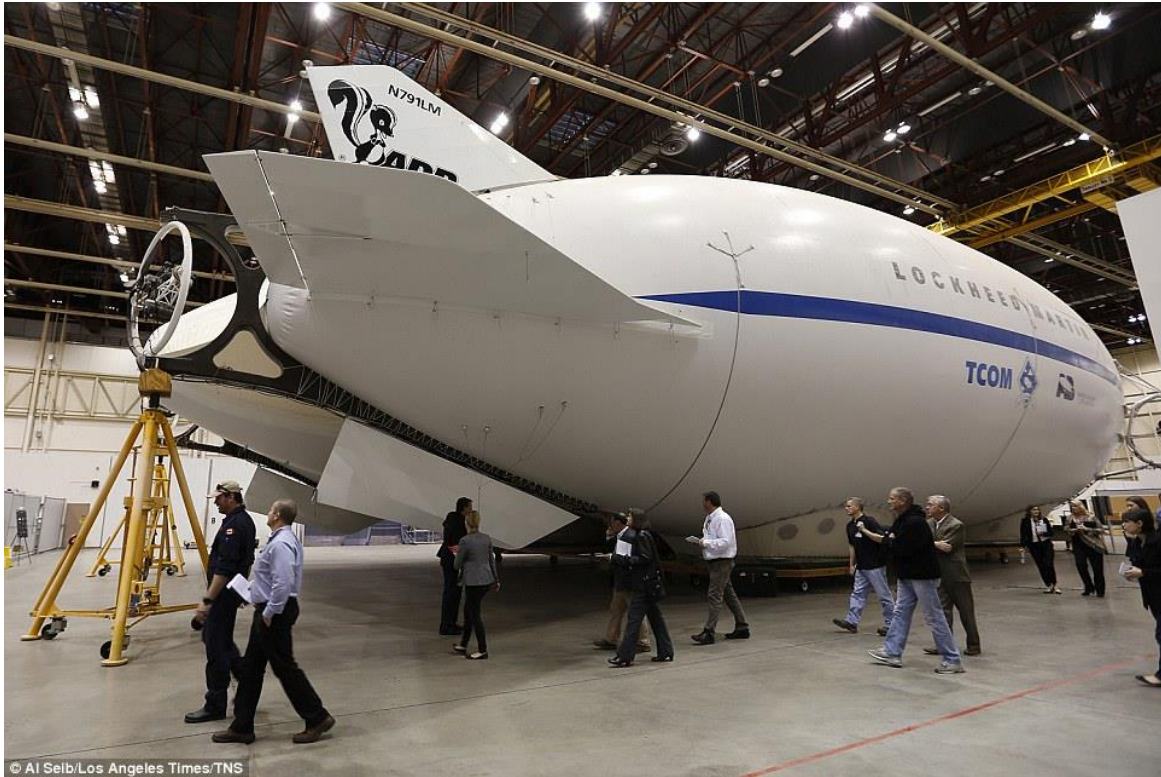
Stern quarter view showing the rear fins and one of two stern vector thrust units. Source: Al Sieb / Los Angeles Times / TNS
