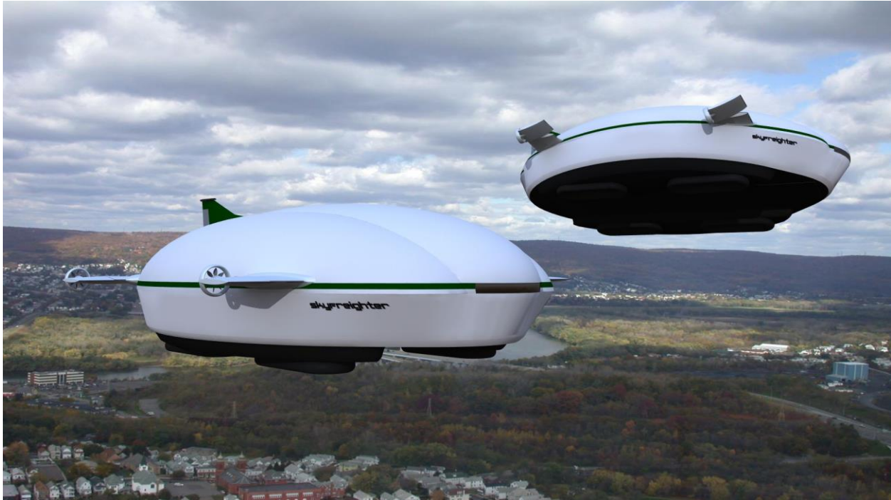
Rendering of two SkyFreighter SF50T airships in flight, with ThrustWings in cruise position (left) and vectored (right). Source: MAS
