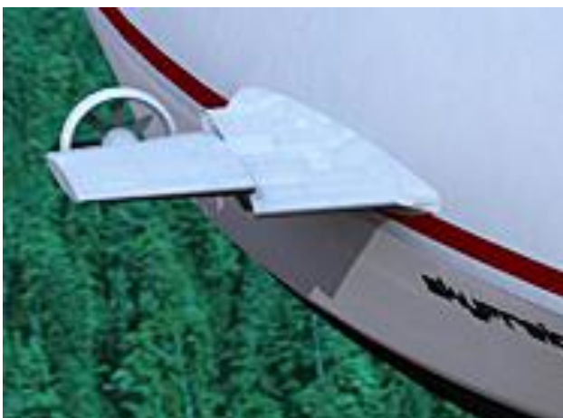
ThrustWing showing the fixed inner stub wing and movable outer section with the propulsor. Source: MAS
