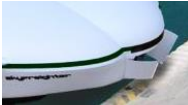
Bow loading doors. Source: MAS
