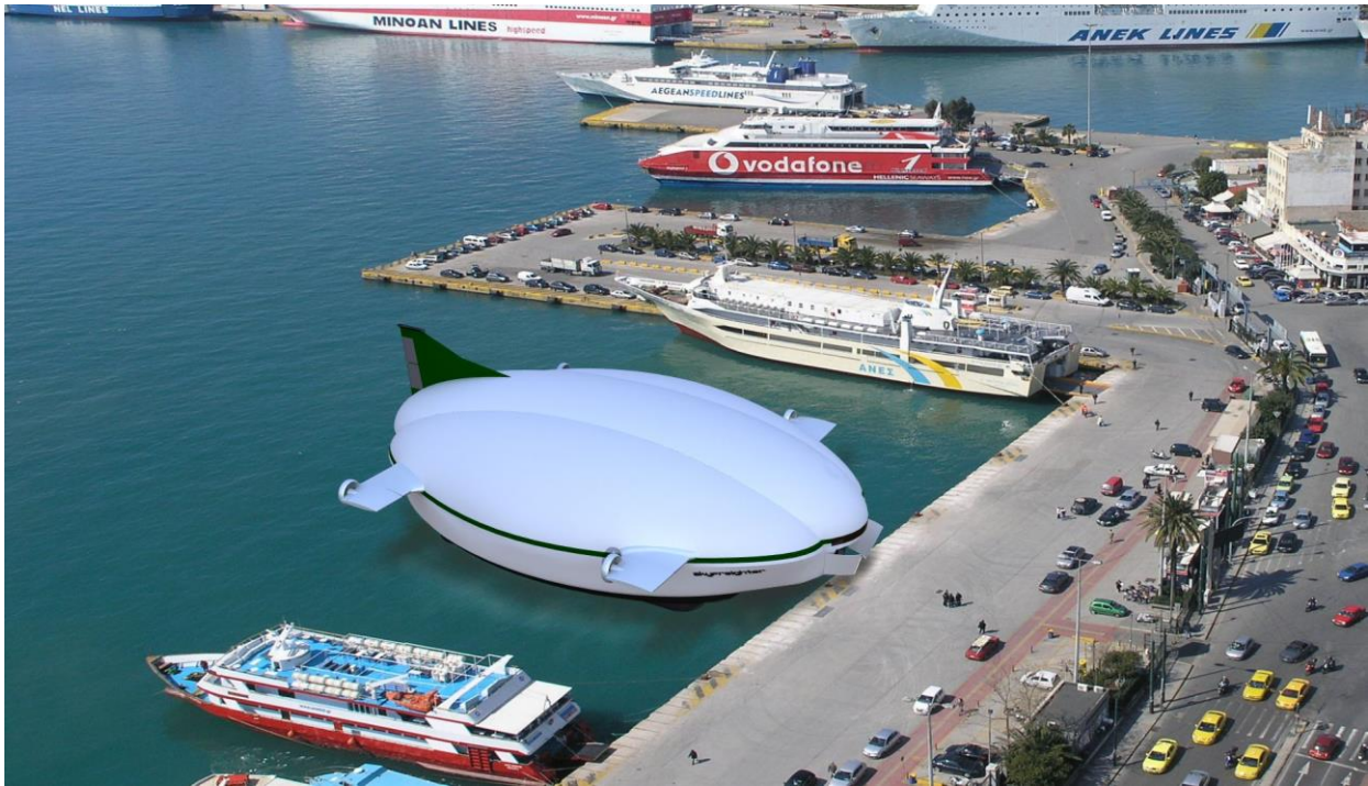
Rendering of a SkyFreighter SF50T airship dockside, loading and unloading from a bow door. Source: MAS
