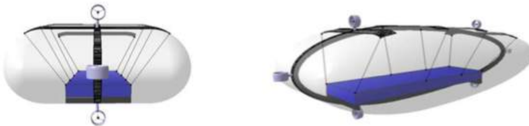
Eletttra Twin Flyers monohull (the "third design") showing details of the exoskeleton. Source: Cappadona, Lecca, Vazzola, Gili, Farina & Surace, 2009
