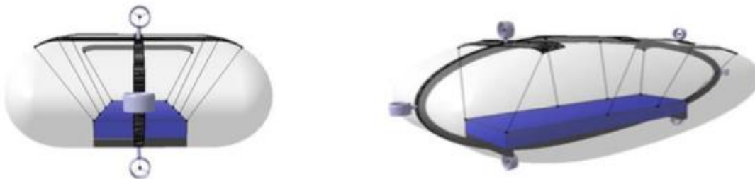
Elettta Twin Flyers monohull (the "third design") showing details of the exoskeleton. Source: Cappadona, Lecca, Vazzola, Gili, Farina & Surace, 2009
