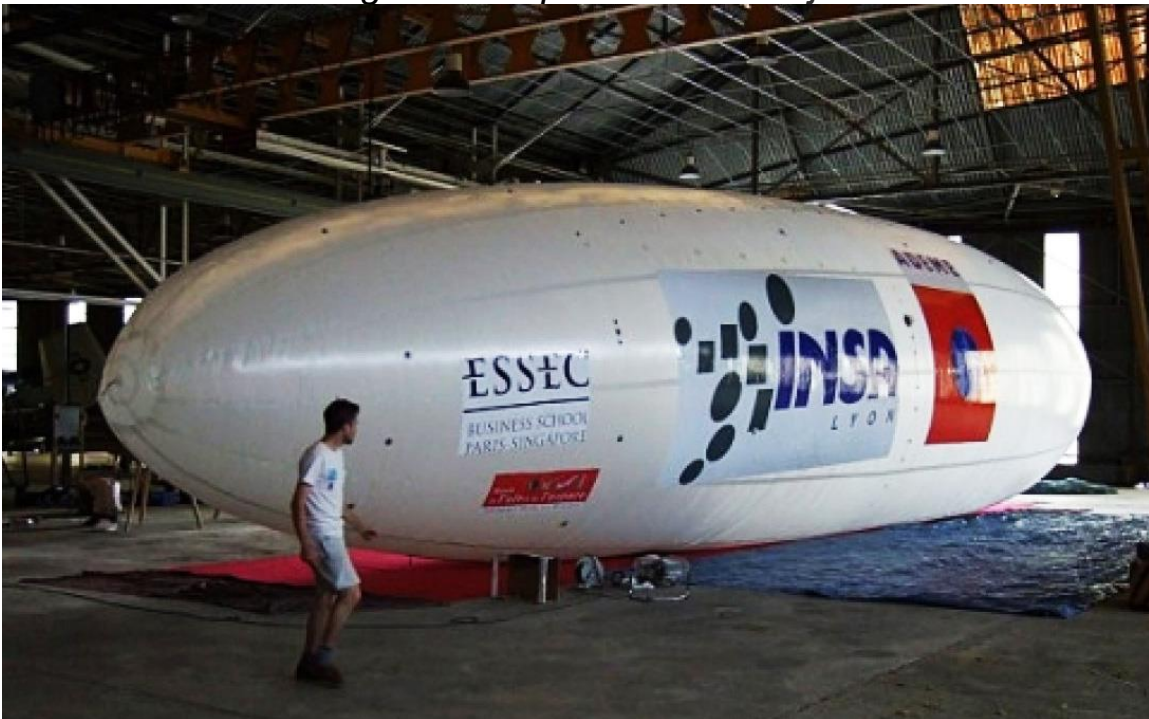
The gas envelope in a hangar, ready for flight. Source: Project Sol'R
