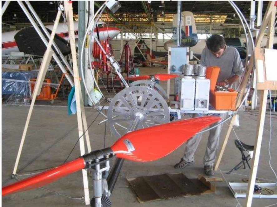
One propeller and drive assembly. The battery is in the orange box on the gondola frame. Source: Project Sol'R
