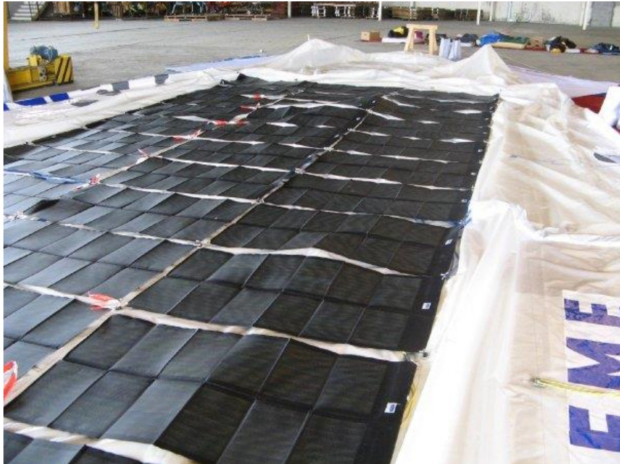
Flexible solar array on the gas envelope. Source: Project Sol'R
