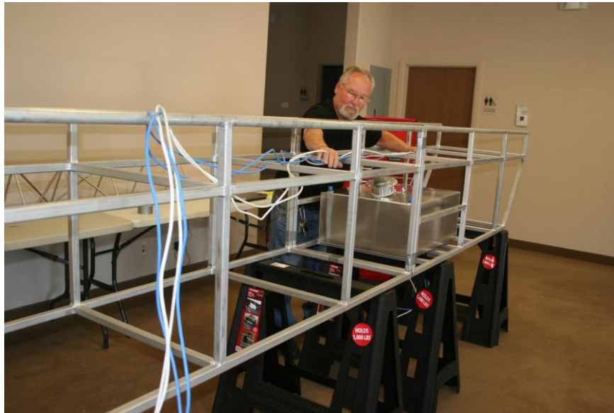
Above: Gondola structure with a fuel tank being installed. Below: Another view of a gondola assembly. Source: Airship Manufacturing via New Atlas
