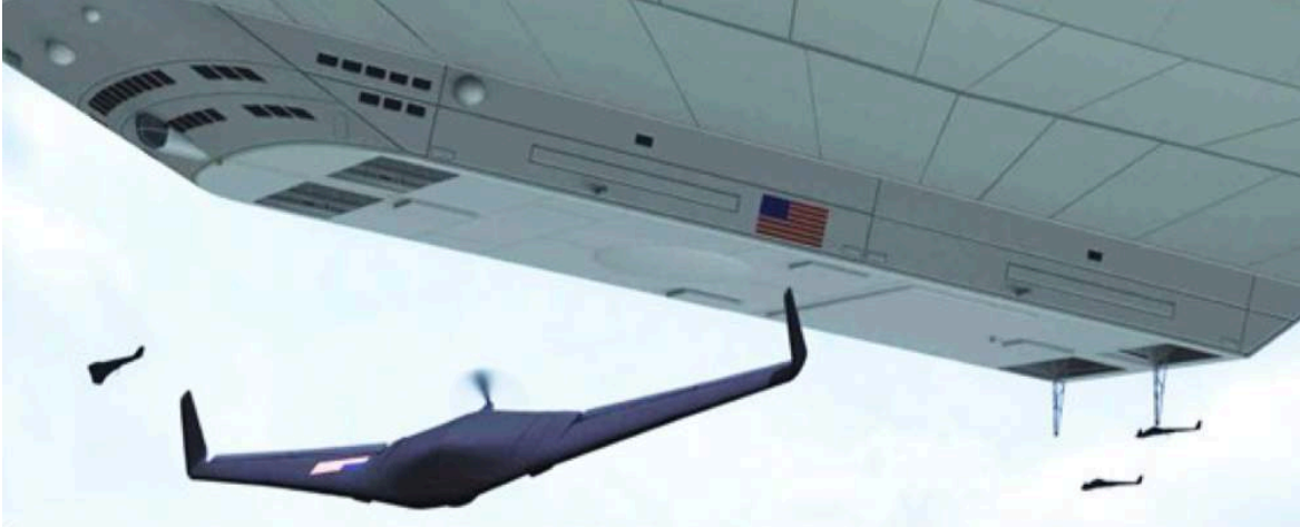
Close-up view of UAV launch (forward bays) & recovery via trapeze (aft bays). Source: SAIC, graphics by Faisla Ali & Pat Rawlings
