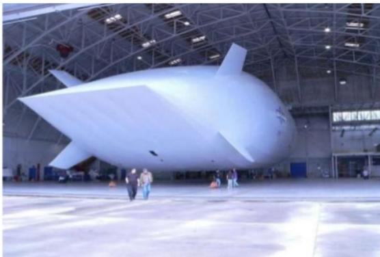
Helium retention was a problem for the Stratellite One, and Sanswire investigated new materials to help minimize helium loss. By 2007, no flight tests had occurred. Work on Stratellite One was abandoned at about this time. The prototype was dismantled and the aluminum frame was sold as scrap.
