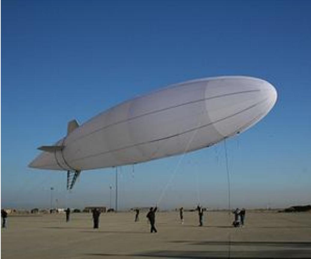
*Sanswire 2A Technology Demonstrator tethered test.
