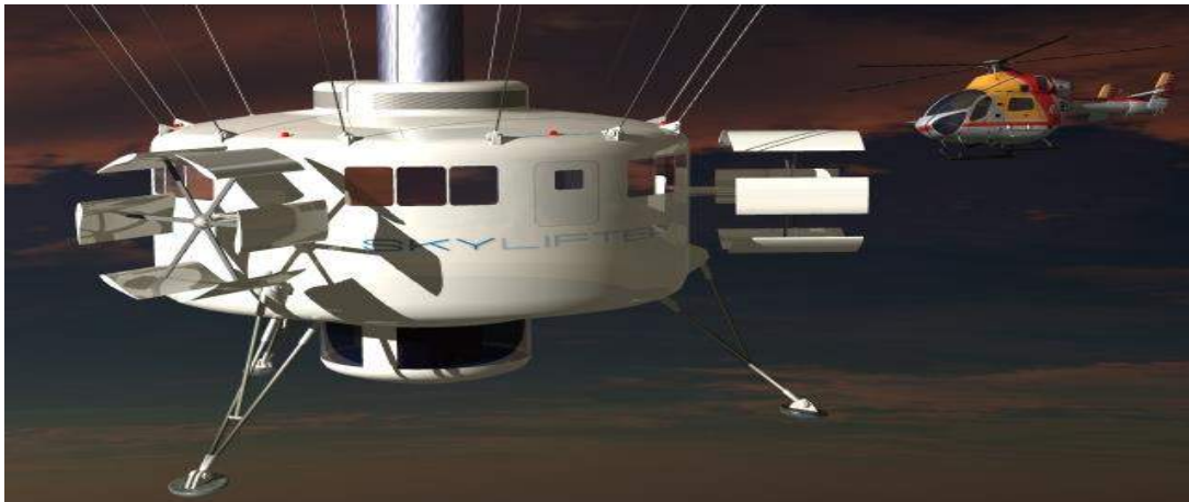
SkyLifter SL150 control pod. Note the attachment points for the suspension lines from the aerostat and the landing legs.
