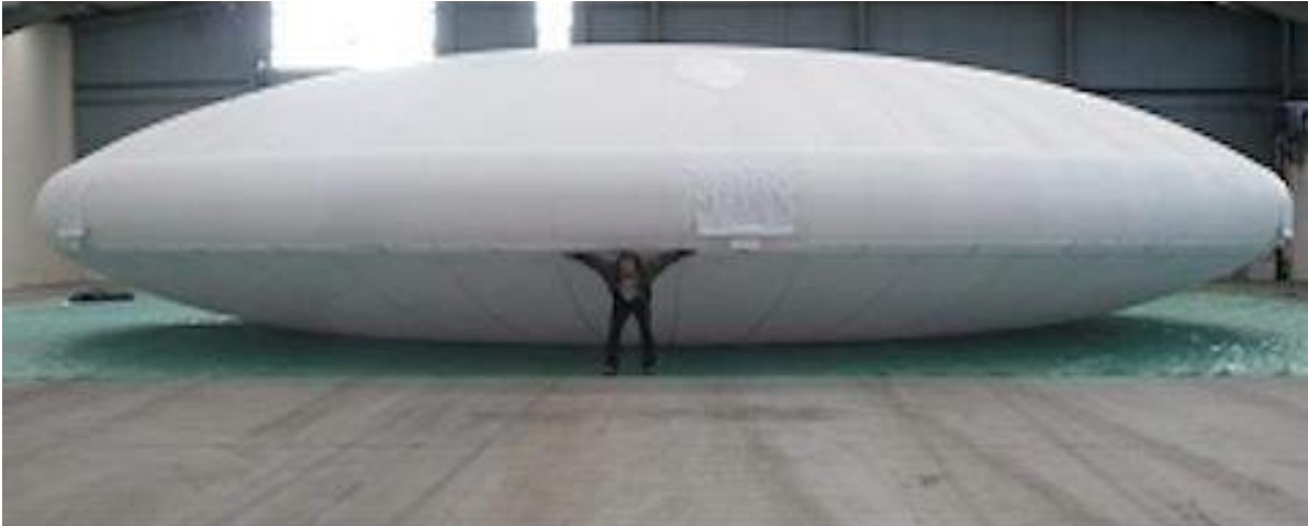
Vikki concept demonstrator with 18 m (60 ft) diameter lifting envelope. Source: SkyLifter Ltd.
