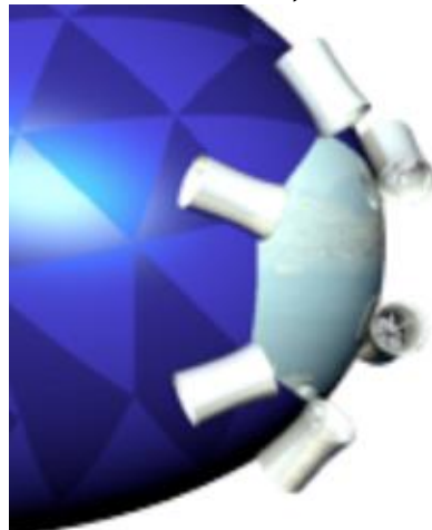
Bow ducted fan thruster array. Source: Skylite Aeronautics
