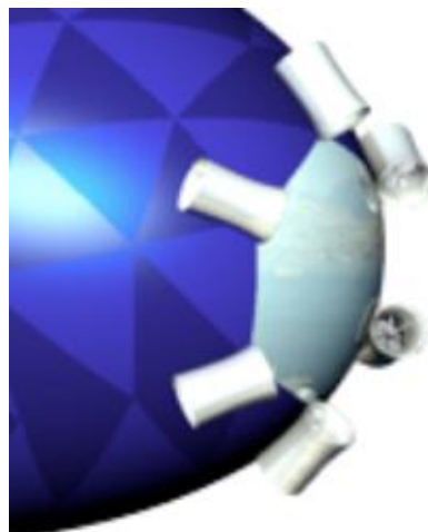
Bow ducted fan thruster array.
