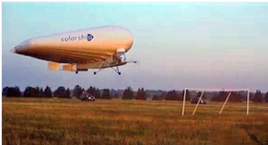
20-m Caracal prototype during the 2014 soccer field test. Source: Screenshot from Solar Ship video
