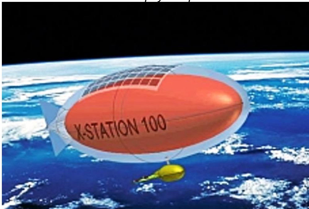
A double-skinned balloon carries the small payload plane to a geostationary position on the stratosphere. Source: StratXX
