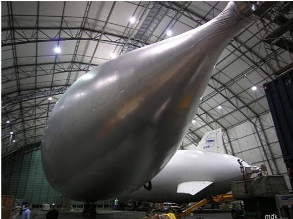
*18,000 m<sup>3</sup> (635,664 ft<sup>3</sup>) X-Station prototype in the Zeppelin Hangar in Friedrichshafen, Germany, along with a Zeppelin NT (background).*
