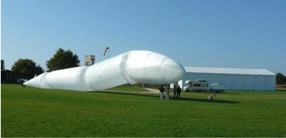
STS-111 mid-altitude, long-endurance UAV segmented airship shown on the ground in 2009. Source: Sanswire-TAO
