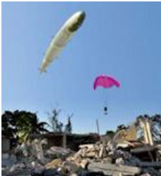
Rendering showing emergency supplies being dropped from SkyDragon using ALF for pinpoint delivery. Source: TAO Group.
