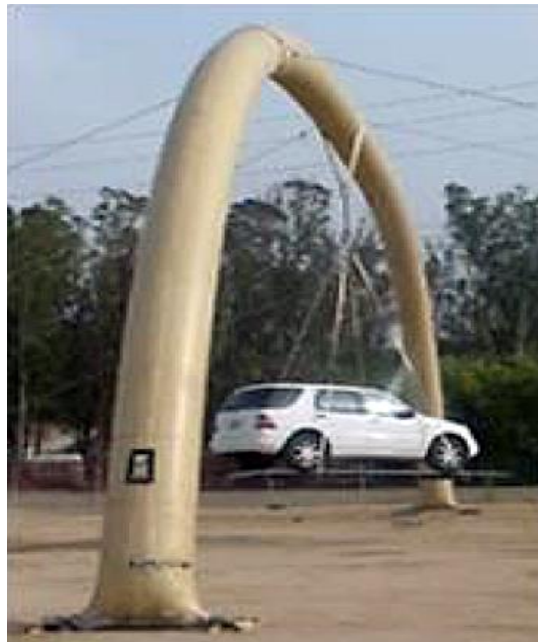
TP Aerospace airbeam suspending a car. Source: NASA Ames Research Center, June 2016
