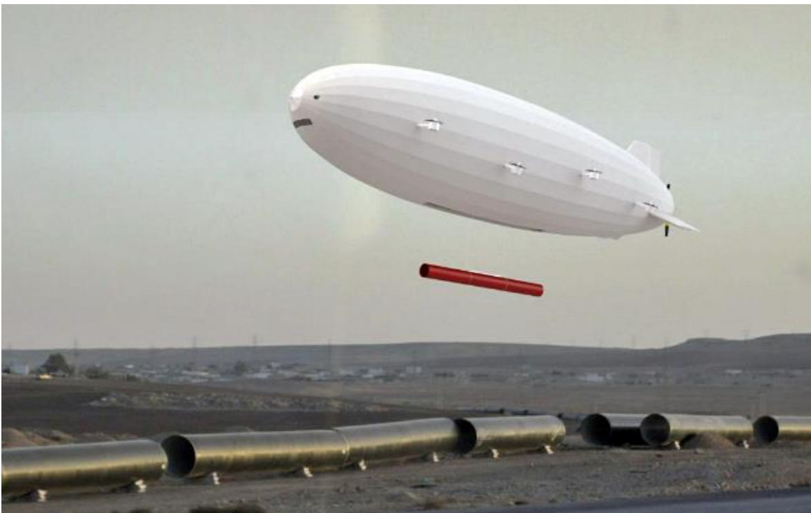
Two renderings of an Atlas 80 operating as a flying crane carrying a large external load. Source: TP Aerospace, Inc.
