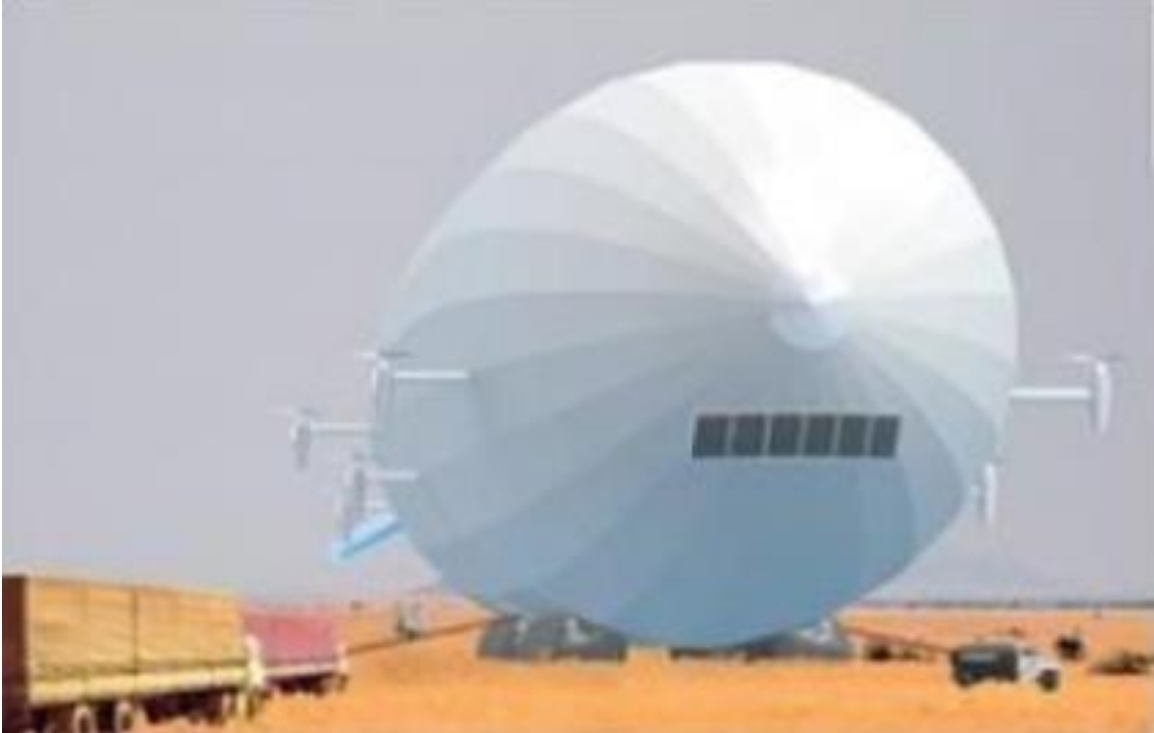
Concept drawing showing an Atlas 80 on the ground at an austere site unloading via side cargo doors. Source: TP Aerospace, Inc.
