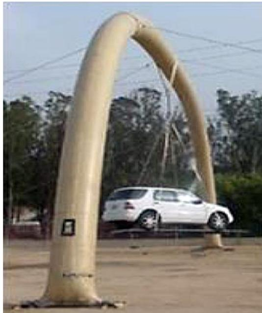
*TP Aerospace airbeam suspending a car.
