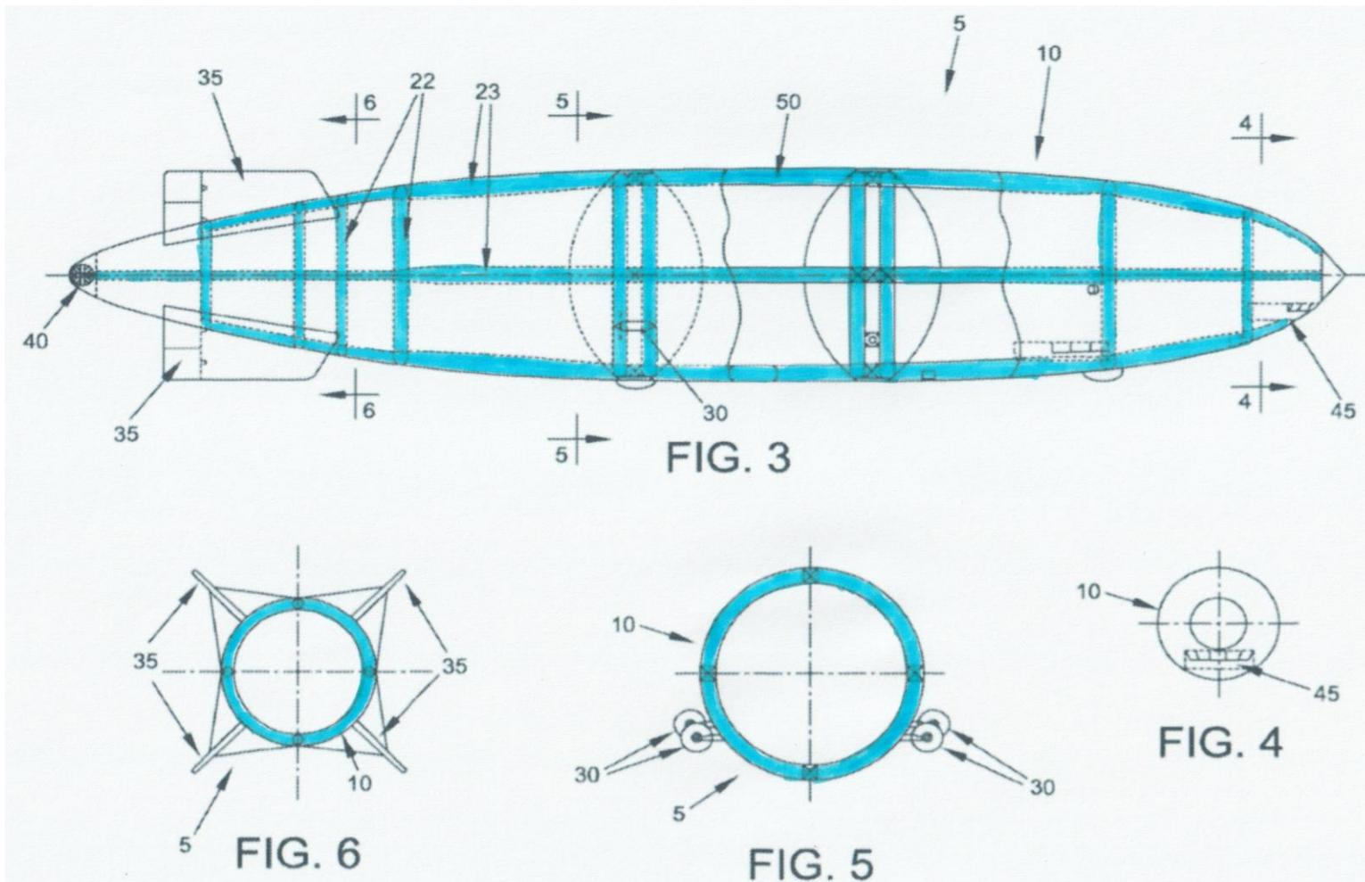
*This is an alternate design of a rigid airframe (15) with high-pressure inflated structural tubes (50). The rigid airframe, highlighted in blue, is comprised of circular hoop sections (22) and longitudinal strut sections (23) laid out in a different configuration than in patent Figures 1 and 2. Two closely spaced circular hoop sections reinforce the hull where the engines (30) attach.*
