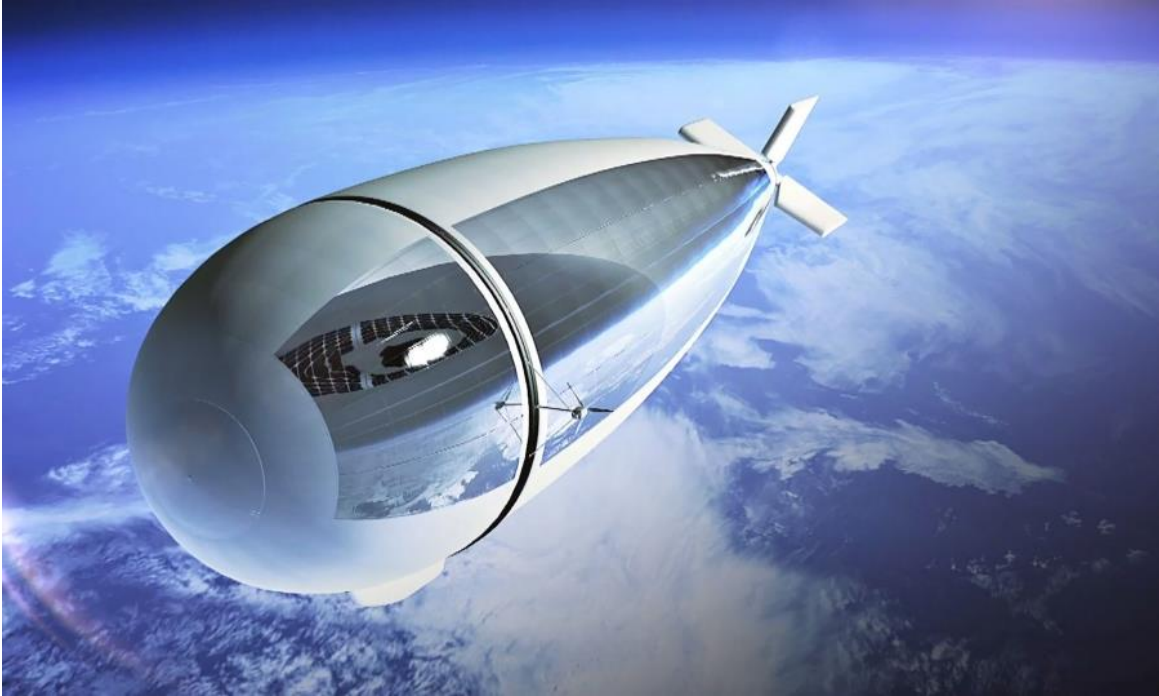
Above: Stratobus with the transparent section of the envelope rotated to improve solar power generation at low sun angles.
