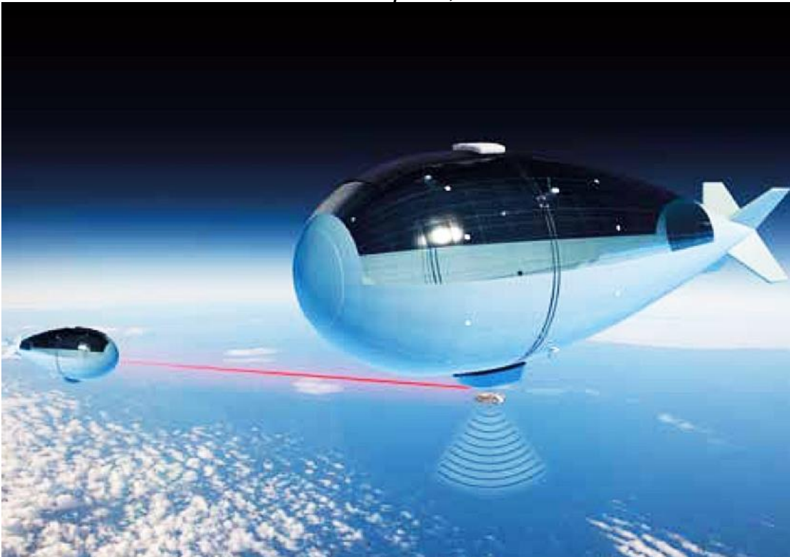
Below: Stratobus showing air-to-ground wireless and airship-to-airship laser data links. Source, both graphics: Thales Alenia Space, circa 2016
