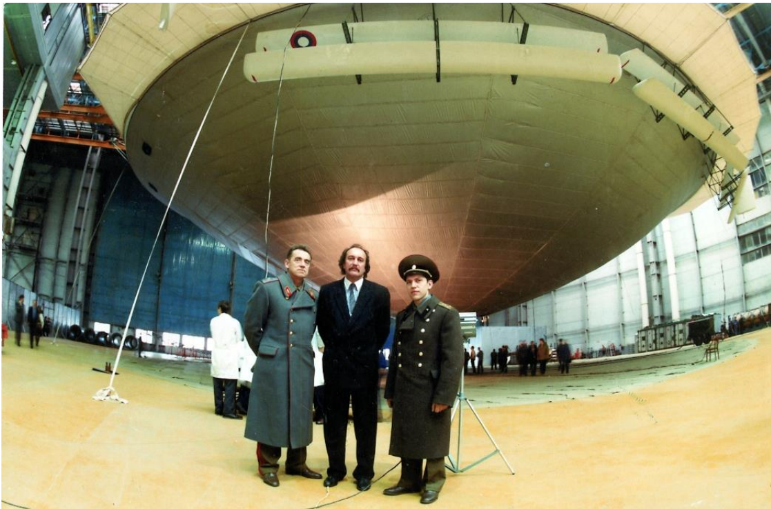
Wide-angle view of the ALA-40-01 and dignitaries posing under the stern of the airship. Note the extended equatorial fairing above the control surfaces. Source: http://topsecretairplanes.blogspot.com/
