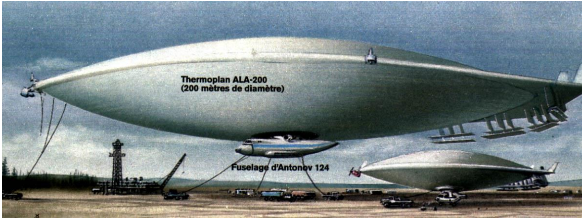
Rendering of the ALA-200 & ALA-40, with the fuselage of an An-124 transport aircraft as the ALA-200's gondola. Source: jb.aeronef
