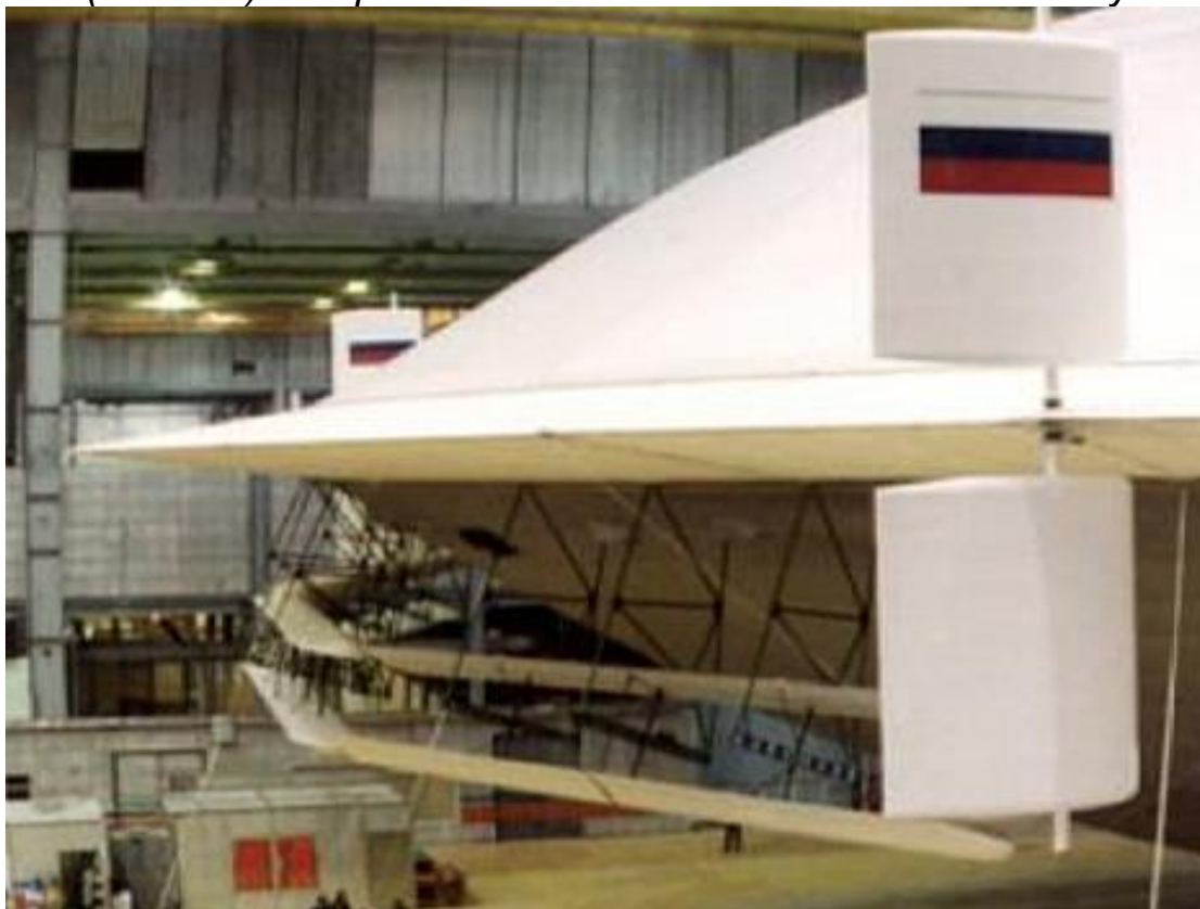
Close-up of ALA-40-01 aerodynamic control surfaces & extended equatorial fairing at the stern. Source: Russian Aeronautical Society
