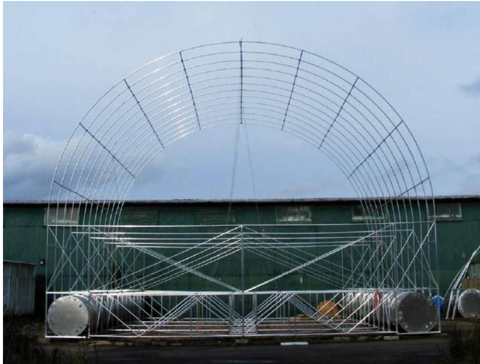
Tubular framework and receiver tanks for one variable lift unit.
