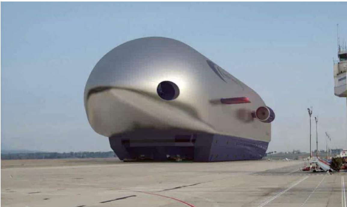
General arrangement of an ARH 50 airship. The cargo deck is the dark structure attached below the aluminum hull. Note the dark lateral thruster ports near the nose and tail and the fixed side-mounted propulsion gas turbine engines. Source, both graphics: Varialift.
