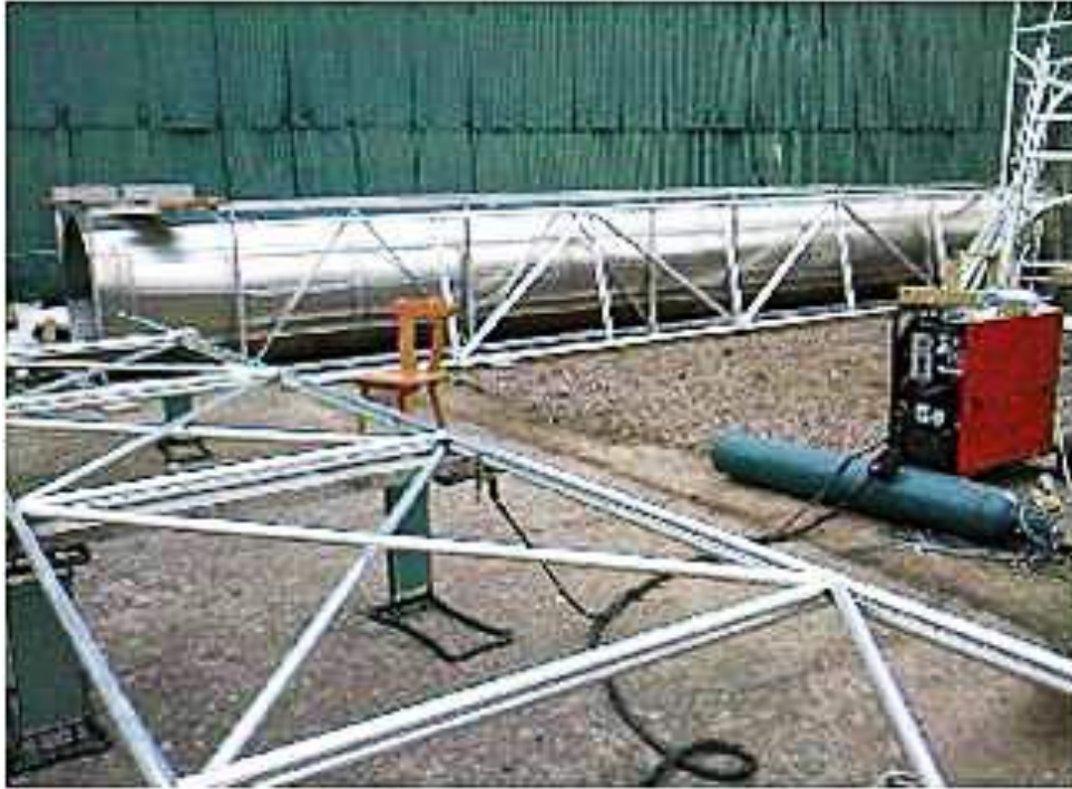
Receiver tank installed in fuselage structure.
