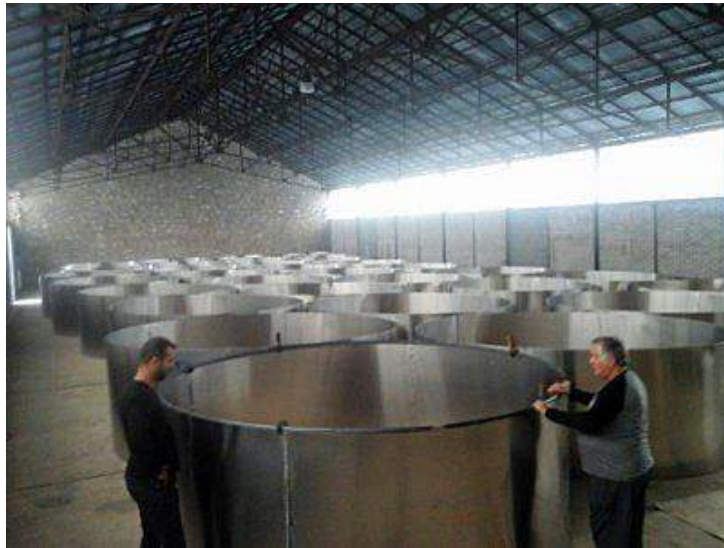
Helium receiver tank segment and end dome manufacturing was underway. Source, both photos: Varialift (circa 2 nd half of 2018)
