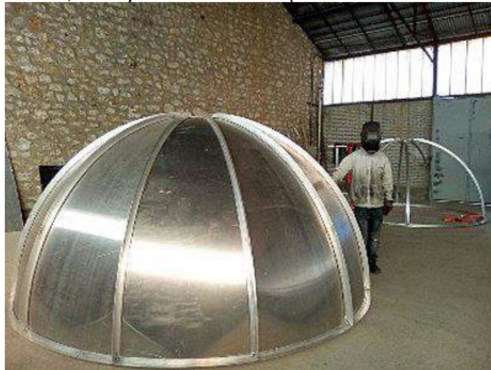
Helium receiver tank segment and end dome manufacturing was underway. Source, both photos: Varialift (circa 2 nd half of 2018)
