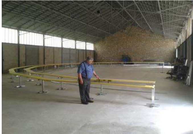
Wooden "jig" on which the semicircular hull frames are built. The frames measure 40 m (131 ft) along the curve; 25 m (82 ft) in diameter. Source: Varialift (circa mid-2017)
