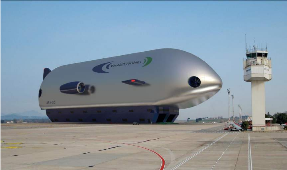
General arrangement of an ARH 50 airship. The cargo deck is the dark structure attached below the aluminum hull. Note the dark lateral thruster ports near the nose and tail and the fixed side-mounted propulsion gas turbine engines. Source, both graphics: Varialift.
