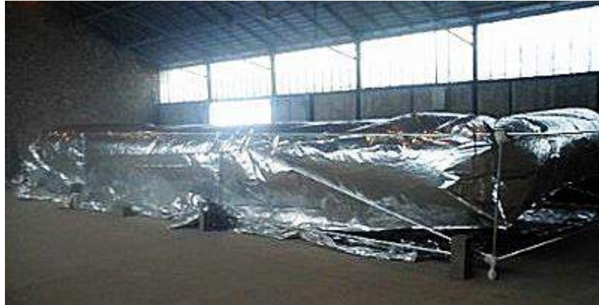
Helium gas cells manufactured & tested. Source: Varialift (circa 2 nd half of 2018)
