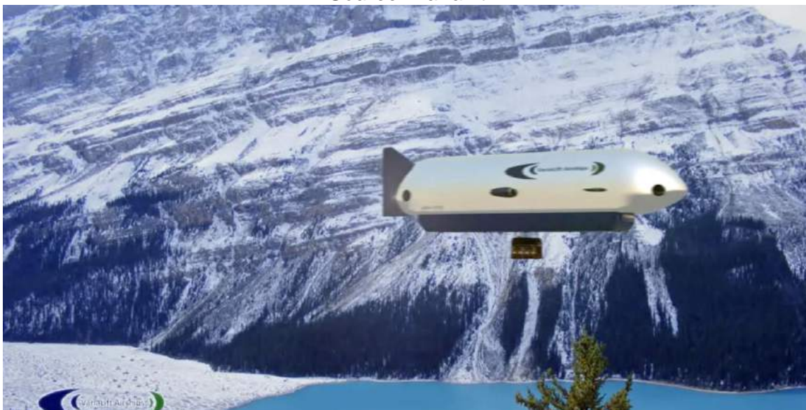
ARH 250 airship transporting a heavy external load. Source: Screenshot from Varialift video.
