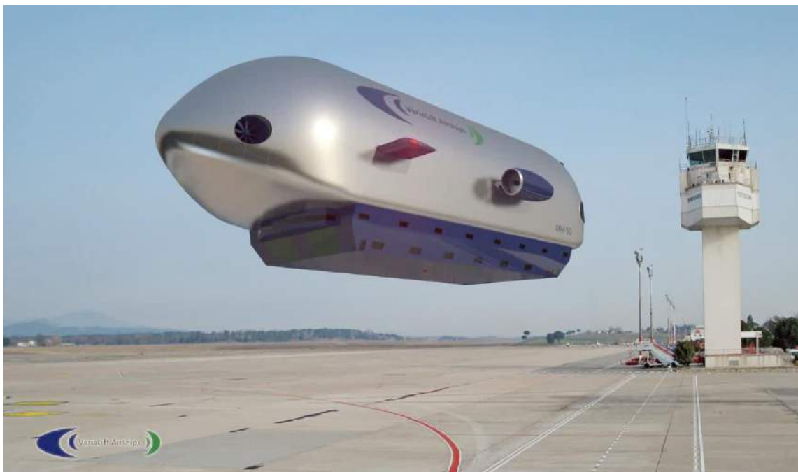
General arrangement of an ARH 50 airship The cargo deck is the dark structure below the aluminum hull. Note the lateral thruster ports near the nose and the side-mounted propulsion gas turbine. Source, both graphics: Varialift.
