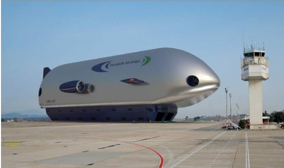
General arrangement of an ARH 50 airship The cargo deck is the dark structure below the aluminum hull. Note the lateral thruster ports near the nose and the side-mounted propulsion gas turbine. Source, both graphics: Varialift.
