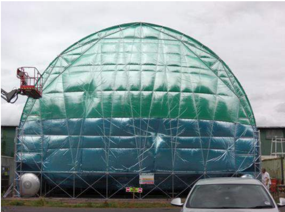
The gas envelope installed in one variable lift unit. Source: Varialift.
