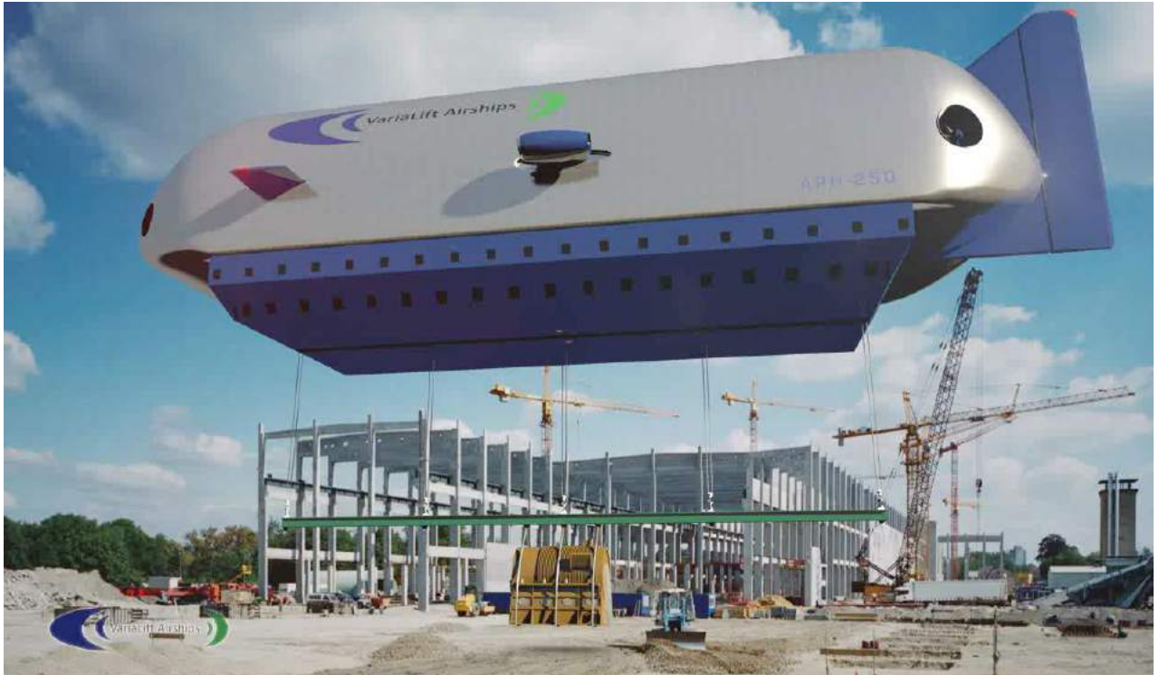
ARH 250 airship hovering and handling heavy external cargo at a remote site. Source: Varialift
