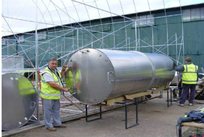
Receiver tank prior to installation in the test rig. Source: Varialift.
