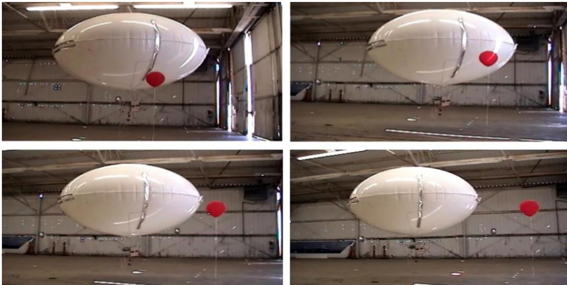
*EK-1 with a skin-integrated propulsion system moving during hanger test flight in 2003. Source: LTAS / Walden Aerospace*
