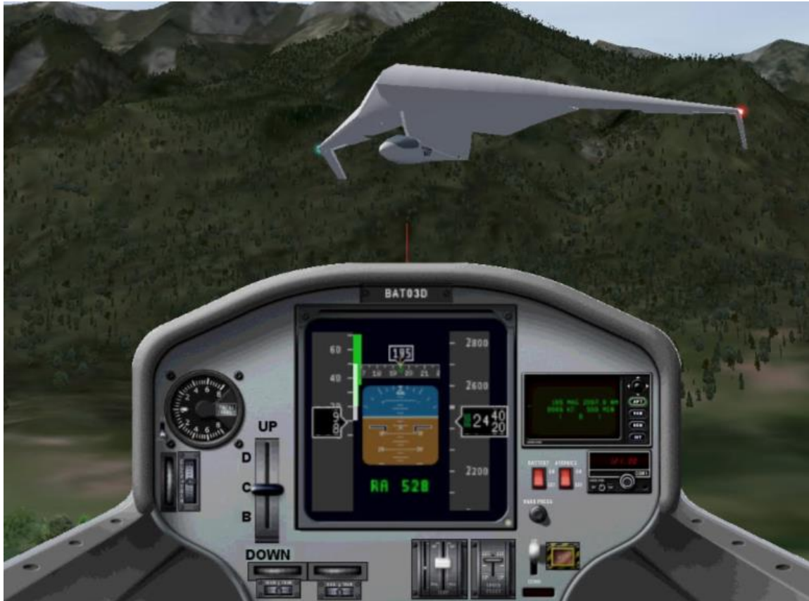
HY-SOAR B.A.T. concept control panel. Note the simple “Up/Down” control for managing buoyancy. Source: Walden Aerospace
