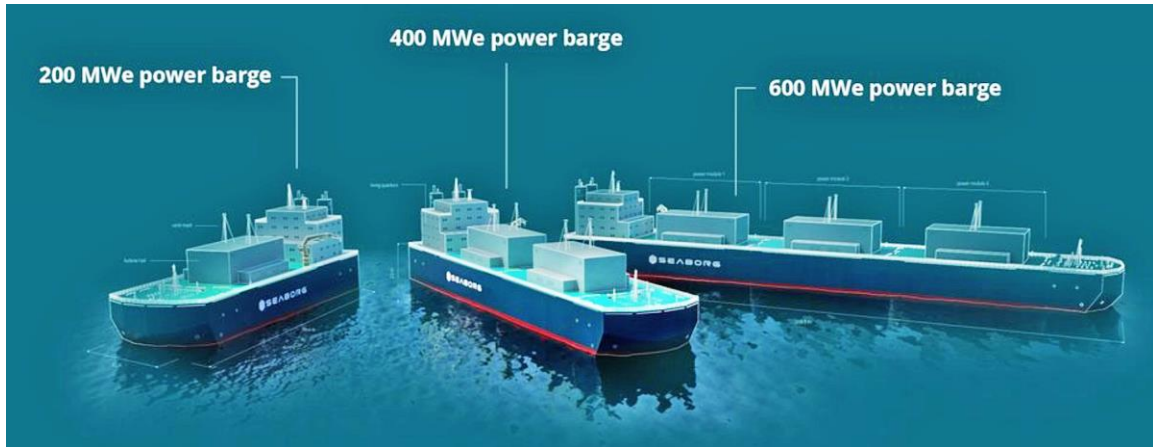
Family of Seaborg power barge with one, two and three power modules. Source: Seaborg Technologies
