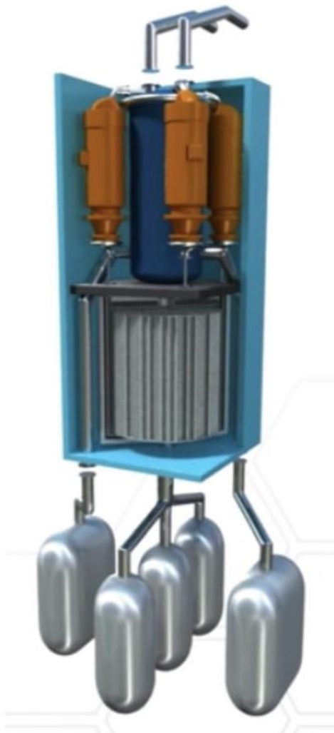
General arrangement of one Seaborg CMSR module showing the heat exchangers (orange) above the reactor, and the drain tanks (silver) under the reactor, design circa 2017. Source: Seaborg Technologies
