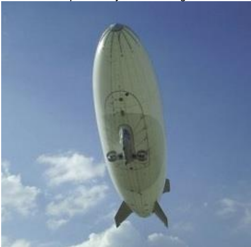
AT-10 flying at Cardington, 31 March 2004. Note the shadow of the single ballonnet on the envelope. Source, both photos: Trevor Monk / Airship Heritage Trust
