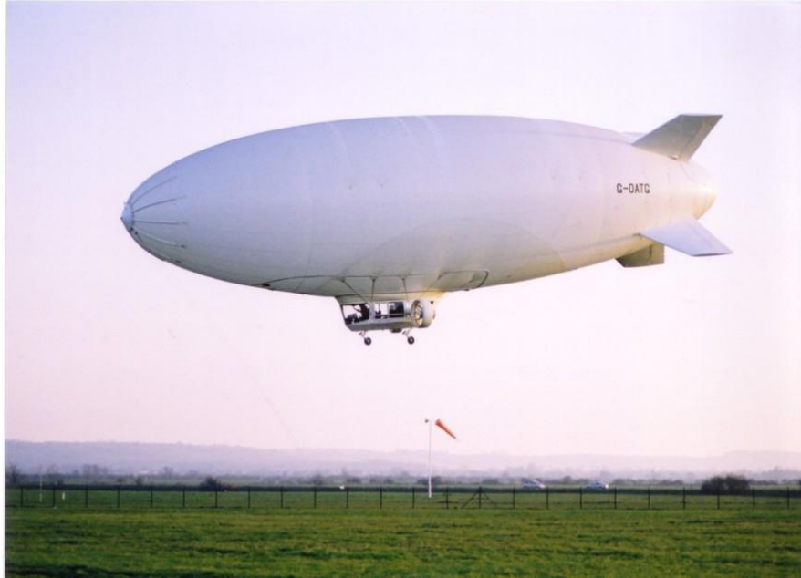
AT-10 in flight. Note the exterior catenary collar and suspension system for the gondola.
