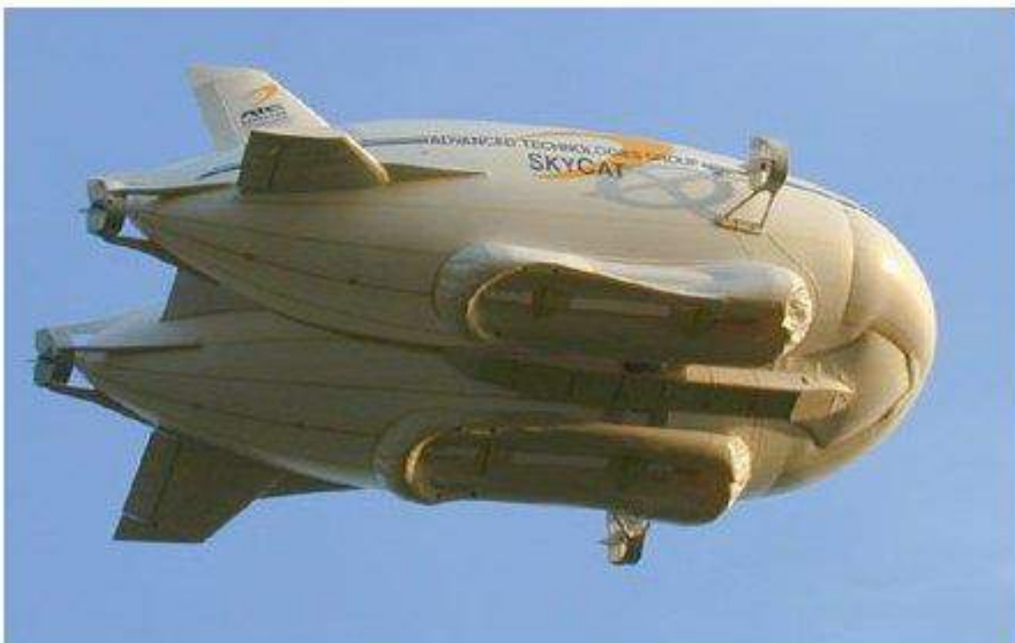
Above: SkyKitten flying overhead showing the air cushion landing system, the central payload pod, and the placement of the four thrust vectoring propulsors. Source: The Airships at Cardington, UK
