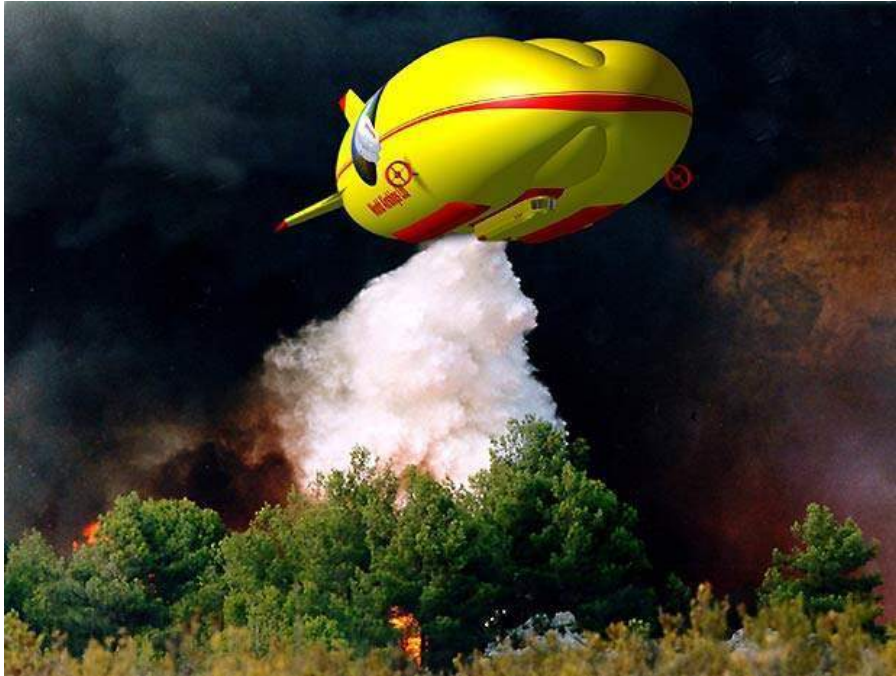
Concept drawing, SkyCat configured as an aerial water tanker to fight forest fires. A water scoop enables the tanker to take water on directly from a nearby body of water. Source: World SkyCat
